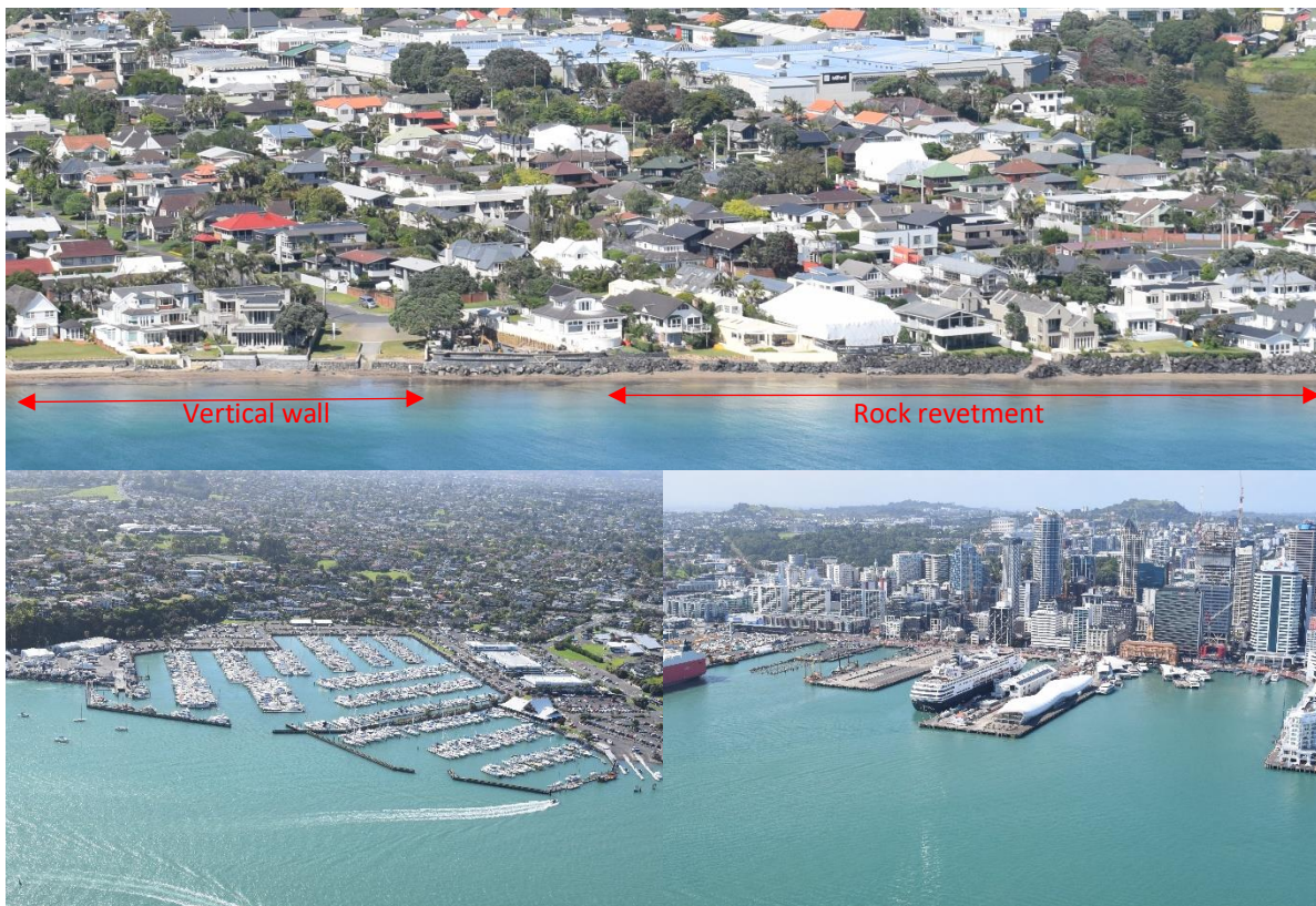
Figure 4.2: Examples of aerial survey photographs used to identify coastal structures such as vertical seawalls and revetments (top panel), marinas (bottom left) and wharfs (bottom right)
