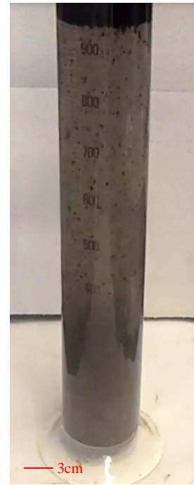
Figure 4.4: The 20 ml HBFO 380 mixture at 15 s showing ~70% of sediment had settled.
