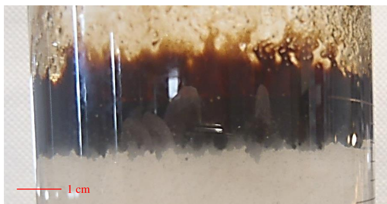
Figure 4.6: The surface portion of oil floating on the seawater surface showing segregated oil droplets situated on the underside.
