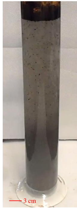
Figure 4.3: The 10 ml HBFO 380 mixture at 15 s showing ~ 70% of sediment had settled.
