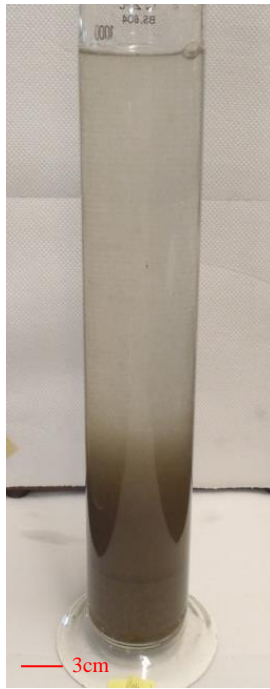
Figure 4.2: the control flask without the addition of oil 15 s after mixing had ceased showing ~30% of sediment had settled.
