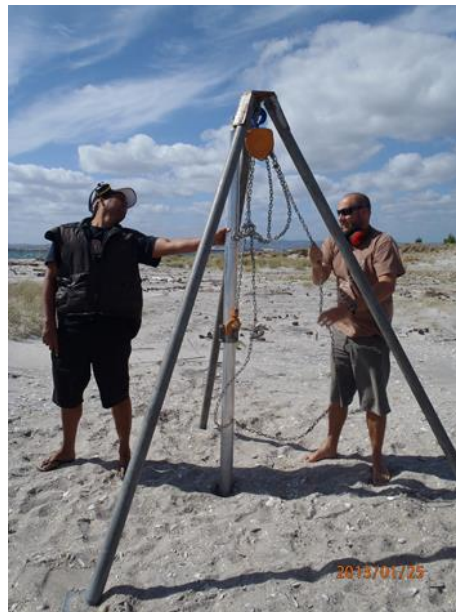
Figure 3.2: the core barrel being winched up on Matakana Island 25th of January, 2013.
