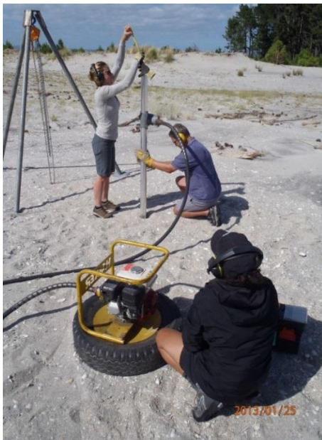
Figure 3.1: Vibrocoring on Matakana Island, 25th of January, 2013.
