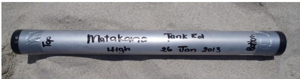
Figure 3.3: Photo of a core cut, capped and taped, ready for transport.
