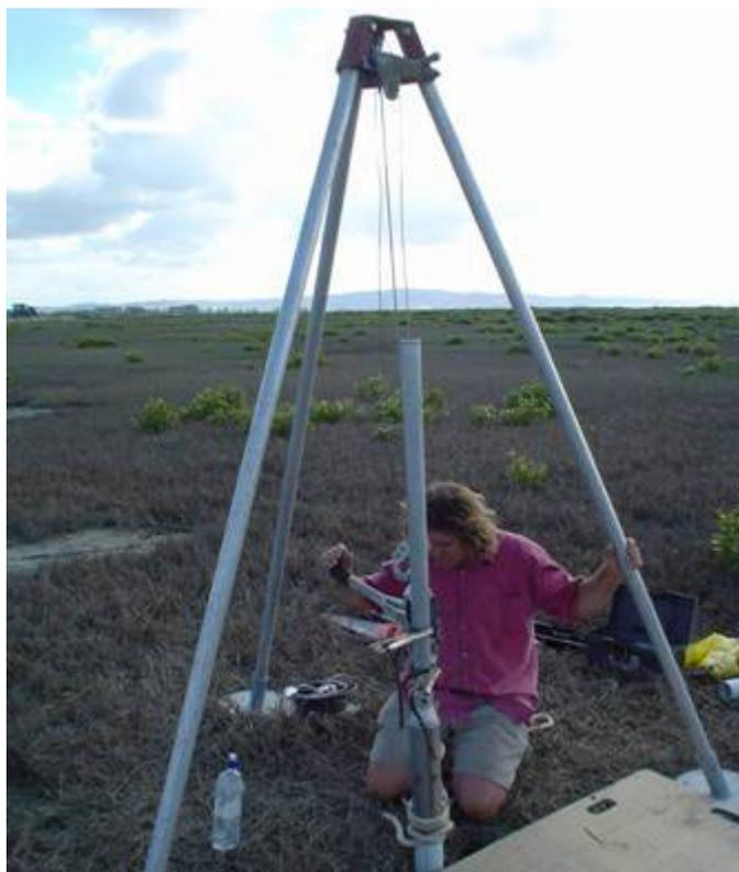
**Figure 3.2:** Sediment coring at site LC-2. Cores are collected in PVC pipe using a Livingston piston corer. The core is extracted from the sediment column using a winch.
