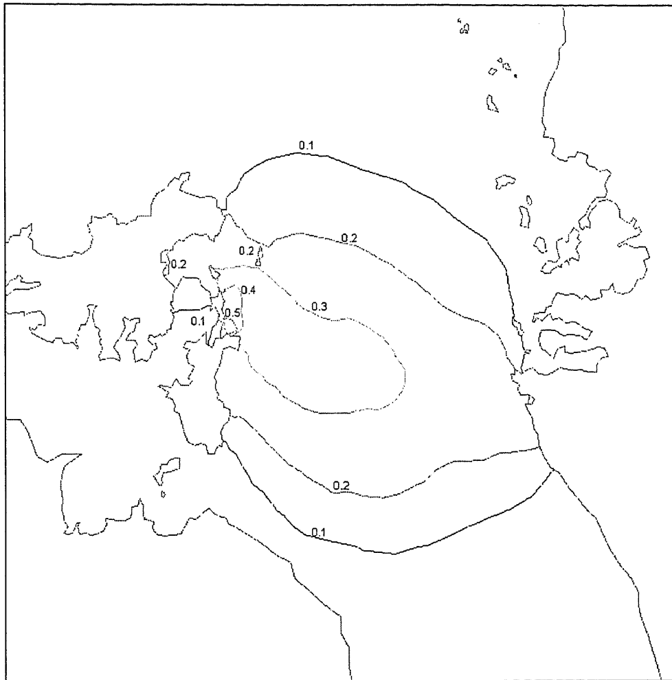
Figure A9.56: Wave height (m) 5 min. 10 s after a 7.35 m displacement along segment D2.
