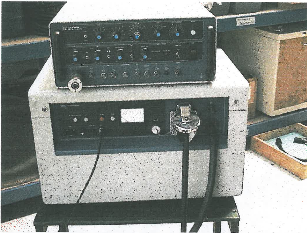
Figure 3.2a: Geopulse model 5210A Receiver sitting upon the Geopulse model 5420A Power Supply.
