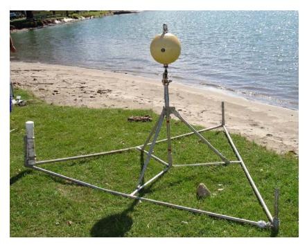
Figure 4.2 The S4 current meter with its frame. Sediment traps were fastened to the sides, as seen to the left of the photo. Photo taken by author.
