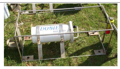
Figure 4.3 The DOBIE water level gauge in an ocean frame. Photo taken by author.
