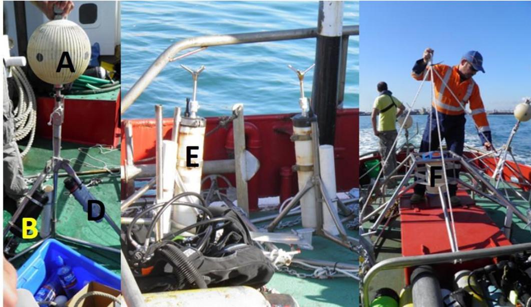
Figure 5 –1 Instruments and equipment used for hydrodynamic and turbidity measurements during this project: (A) InterOcean S4; (B) C3 Fluorimeter, (C) stainless steel frame for mounting instruments; (D) pinger; (E) Acoustic Doppler Velocimeter; and (F) Acoustic Doppler Current Profiler.
