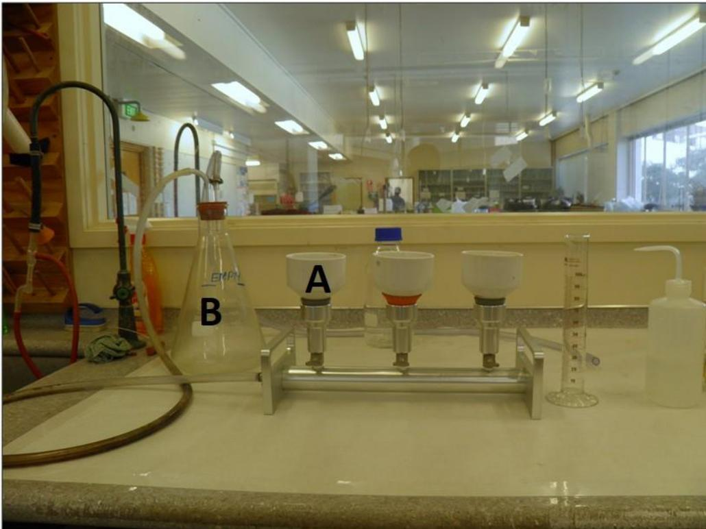
Figure 5-3. Equipment for TSS analysis used in this study. (A) Bucher funnel and (B) Glass flask to collect the filtered water.
