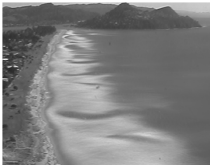
Figure 2. Time-averaged image of Pauanui Beach (North Island, New Zealand) showing large breaking areas (brighter colour) and rip currents (areas where wave breaking does not occur). Localized shoreline erosion is associated with rip currents.
