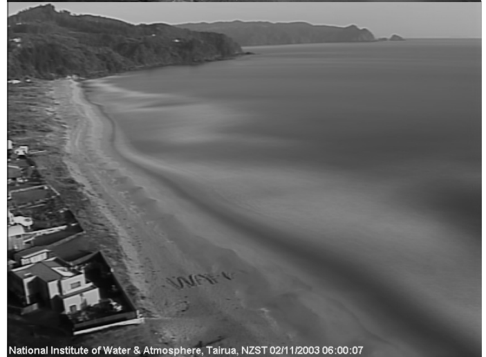
Figure 5. Snapshot (top panel) and time-averaged image (bottom panel) at Tairua Beach (North Island, New Zealand). Time-averaged images are the result of averaging ten minutes of images collected every second (for a total of 600 images). Notice how the shoreline is difficult to characterize on snapshots (top panel) patterns related to individual wave and run-up are discernible. On time-averages (bottom panel) individual run-ups are merged into a shore-break while individual breaking waves are merged around the position of the submerged sandbar.
