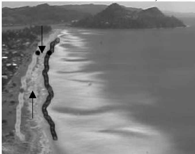
Figure 7. Shoreline and dune detection using a “wet” and “dry” shoreline-detection algorithm. Dark symbols indicate the shoreline, light symbols indicate the edge of the dune. Dark and light filled circles (and arrows) indicate the two locations where beach width was measured.
