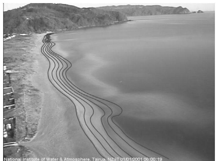
Figure 6. Shoreline detection at Tairua Beach (North Island, New Zealand) using a “wet” and “dry” shoreline-detection algorithm. Shoreline has been detected at different tidal stages resulting in a detailed intertidal bathymetry map.
