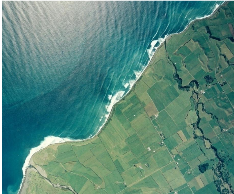
Figure 2.12 Refraction occurring to the north of the Stony River mouth. (Source: TRC, 1995).
