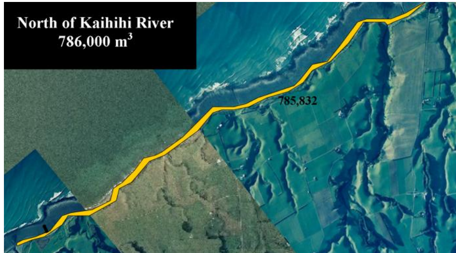
Figure 3.32 Sediment coverage north of the Kaihihi River. The black line shows the location of where the profile was surveyed.
