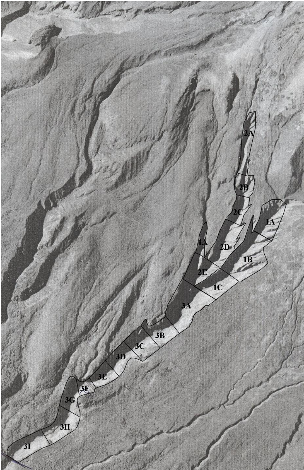
Figure 6.2 The eroded gully in the headwaters of the Stony River (Little Pyramid), divided into segments to determine the cross-sectional area and volume of the material that has been eroded from this scarp.
