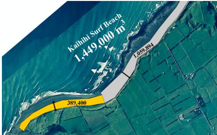
Figure 3.33 Sediment coverage along Kaihihi Surf Beach to the north of the Stony River. The black lines show the location of where the profile was surveyed.
