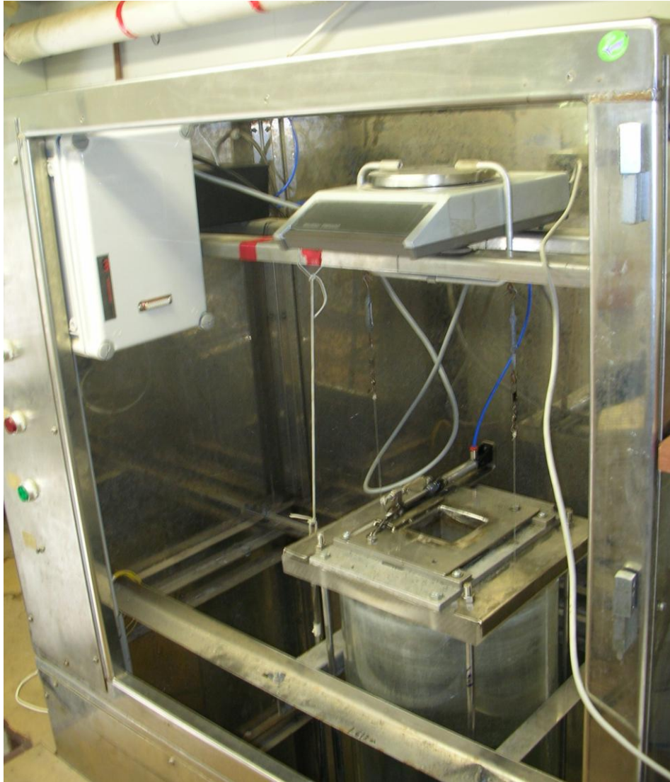
Figure 4.3 The top of the RSA (Rapid Sediment Analyser) at the University of Waikato. (Source: Anais Wille).
