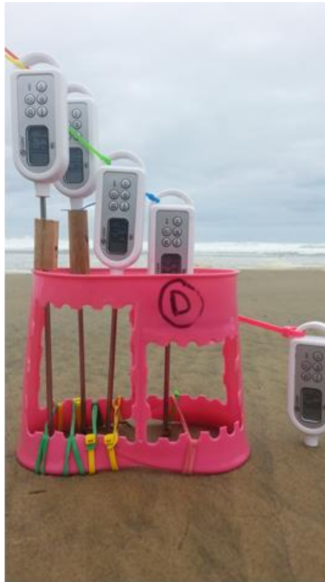
Figure 35: A custom-built thermometer stand allowed for the simultaneous measurement of sediment temperatures at depths of 2 cm, 4 cm, 7.5 cm, 10.5 cm and 20.5 cm below the beach surface.
