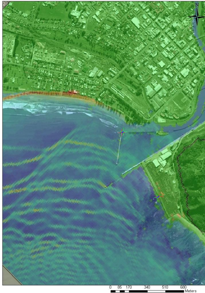
Figure 25 Inundation maps for the city from FAULT B, left shows the wave as it hits and right shows the full extent of inundation for FAULT B (Both images are overlayn on Terralink International 2005 Ltd satellite images)
