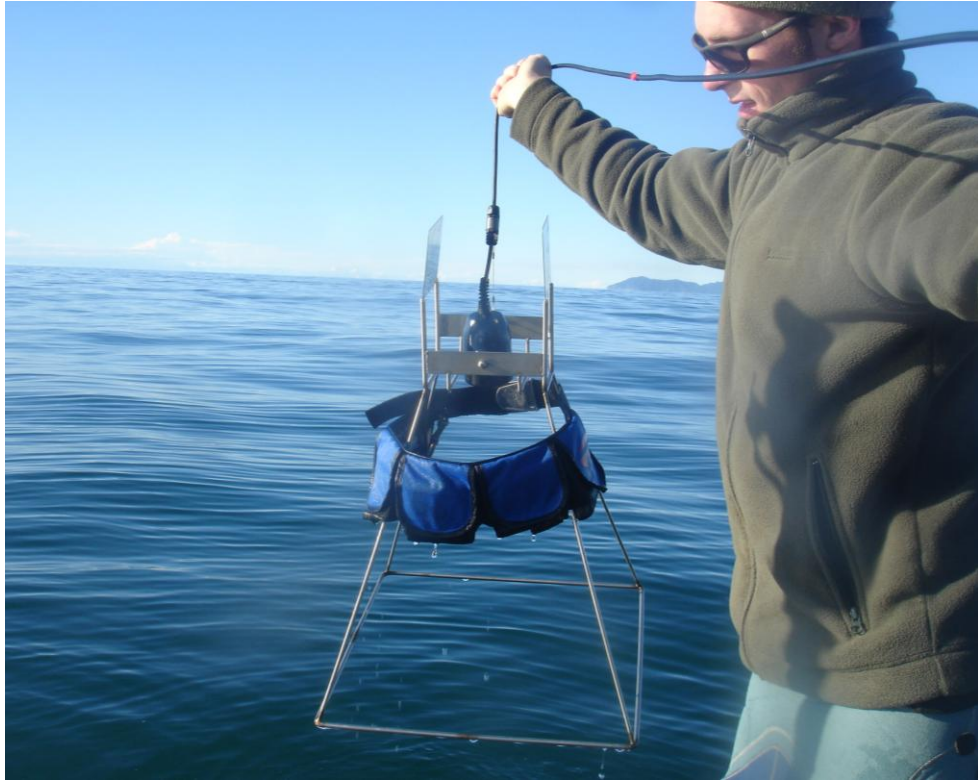
Figure 3.11: The drop-camera attached to a cable and enclosed within a steel frame, with a diving weight belt attached.
