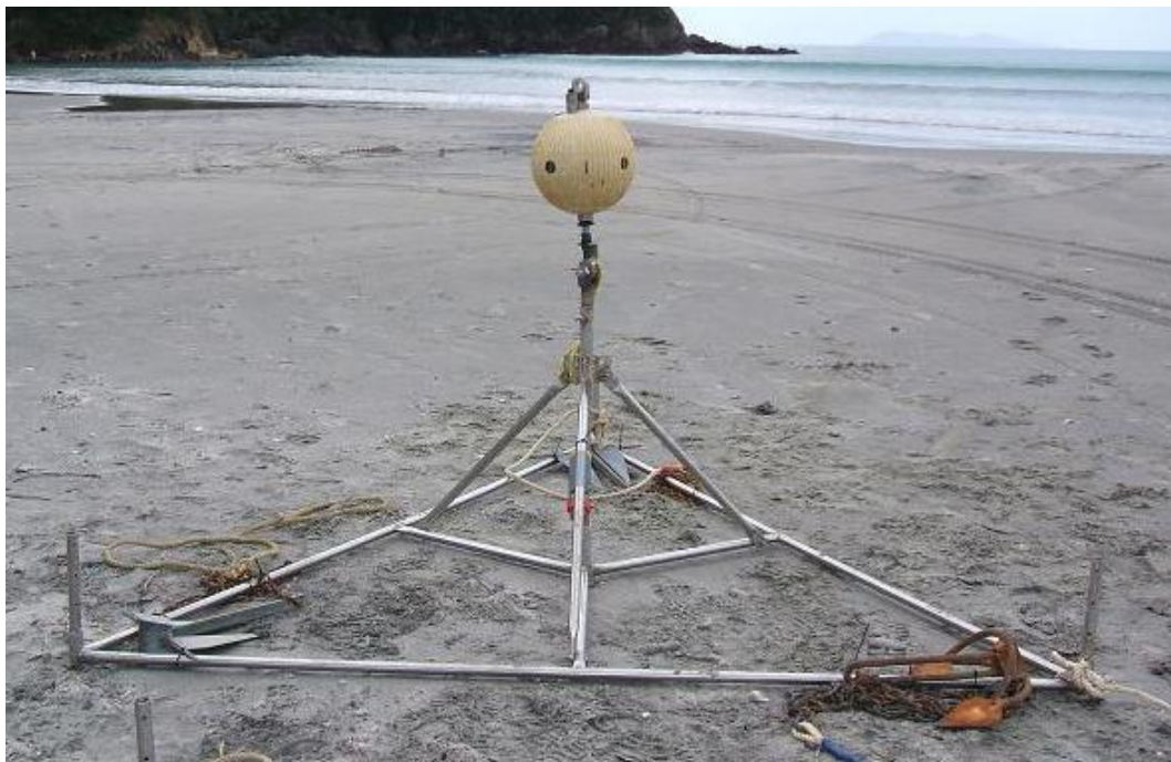
Figure 5.1: S4 current meter mounted on stainless steel tripod.
