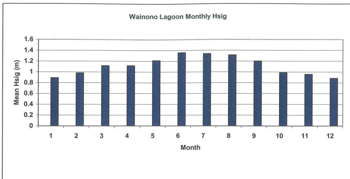
Figure 3.9: Wainono Lagoon monthly significant wave height means at Wainono Lagoon 1979-1998. At 10m depth. Note 1=January 12= December. (Source: NIWA wave hindcast data).
