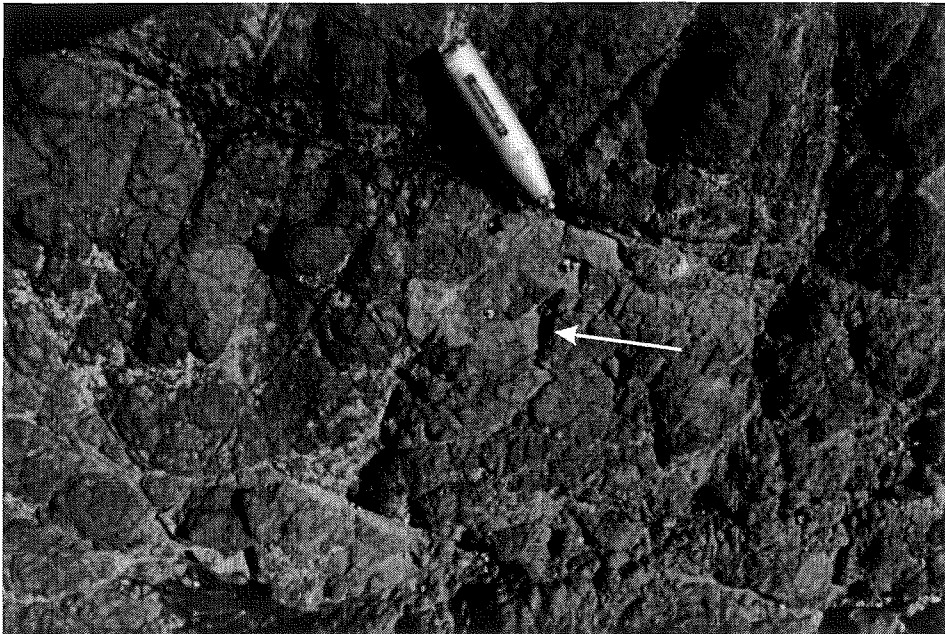
Figure 4.1: Rock surface near AK1D. Showing patterns formed by dominant and secondary fracture planes. Arrow indicates space where block has been removed. Object is 280mm long.
