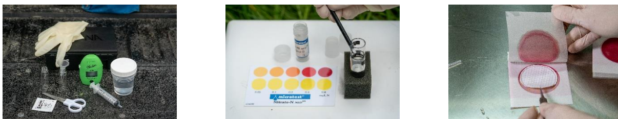
Figure 2-1: Volunteer methods for measuring phosphate (left), nitrate (middle) and E. coli (right) in streams as part of SHMAK.
