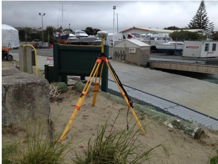
RTK Base Station at BM DML3- Mana Marina
