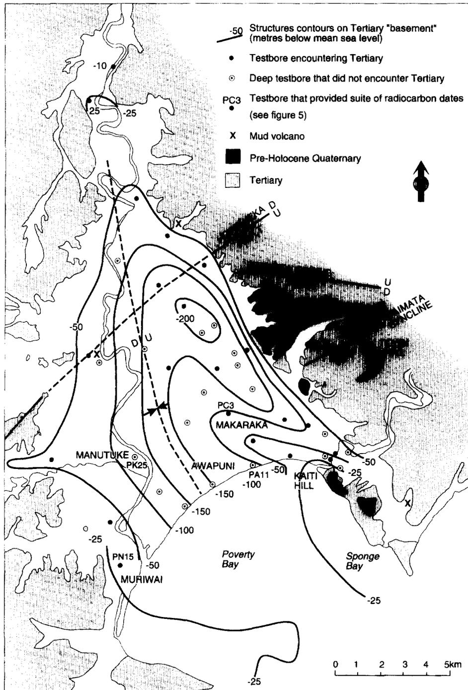
FIG. 3. Structure contours on Tertiary 'basement' beneath Poverty Bay flats and structural features of pre-Quaternary geology.
