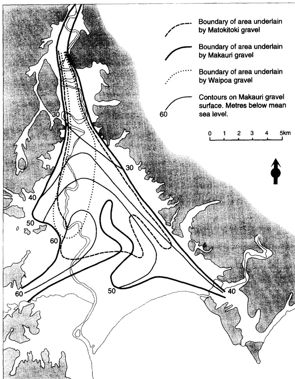
FIG. 4. Fluvial gravel channel deposits underlying Poverty Bay flats and contours on Makauri gravel surface showing tilting to the southwest.
