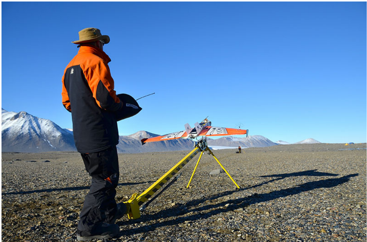
Figure 3.4. UC fixed-wing and slingshot method of launch, featuring University of Canterbury UAV pilot, Paul Bealing, taken in Antarctica (Photo credit: David Risk).
