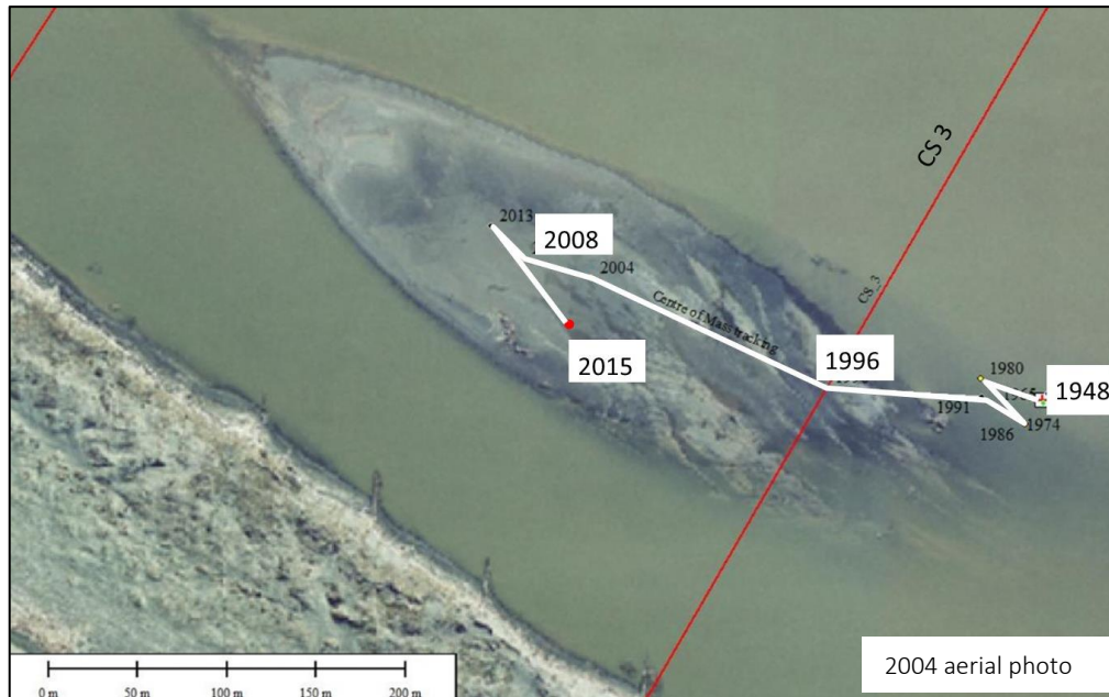
Figure 18 Migration tracking of the Dome-Shoal based on aerial photo centres of mass between 1948 and 2015 superimposed upon the 2004 aerial photograph
