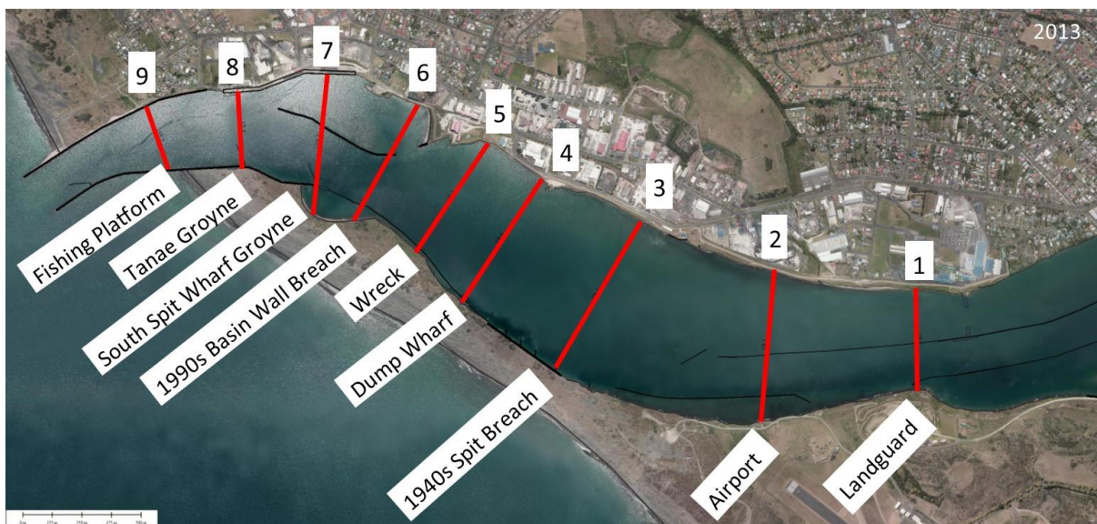
Figure 15 Section locations (red lines), numbers and names superimposed upon a 2013 aerial photograph. Black lines locate river control structures.
