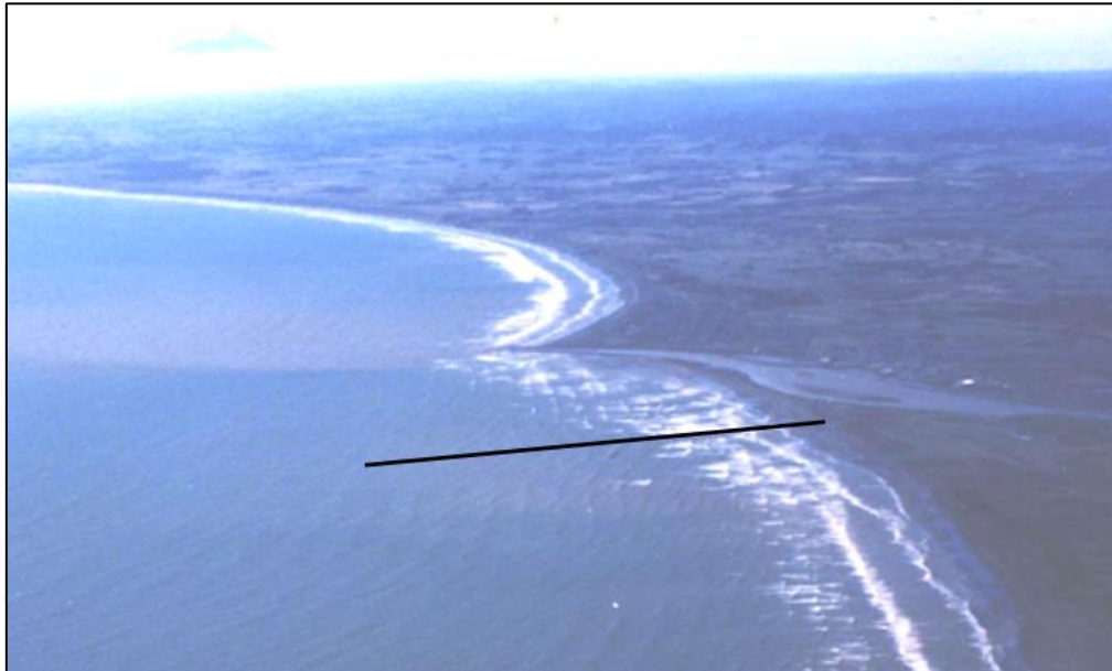
Figure 24 Wanganui coast (1993) with marine outfall (approximately) located. Linear bars and troughs (2D morphology) are evident on the far side of the rivermouth (Castlecliff coast). Two-dimensionality is also evident in bottom of photo (beyond 4 km from rivermouth), with transverse (three-dimensional) morphology from the rivermouth to beyond the marine outfall.
