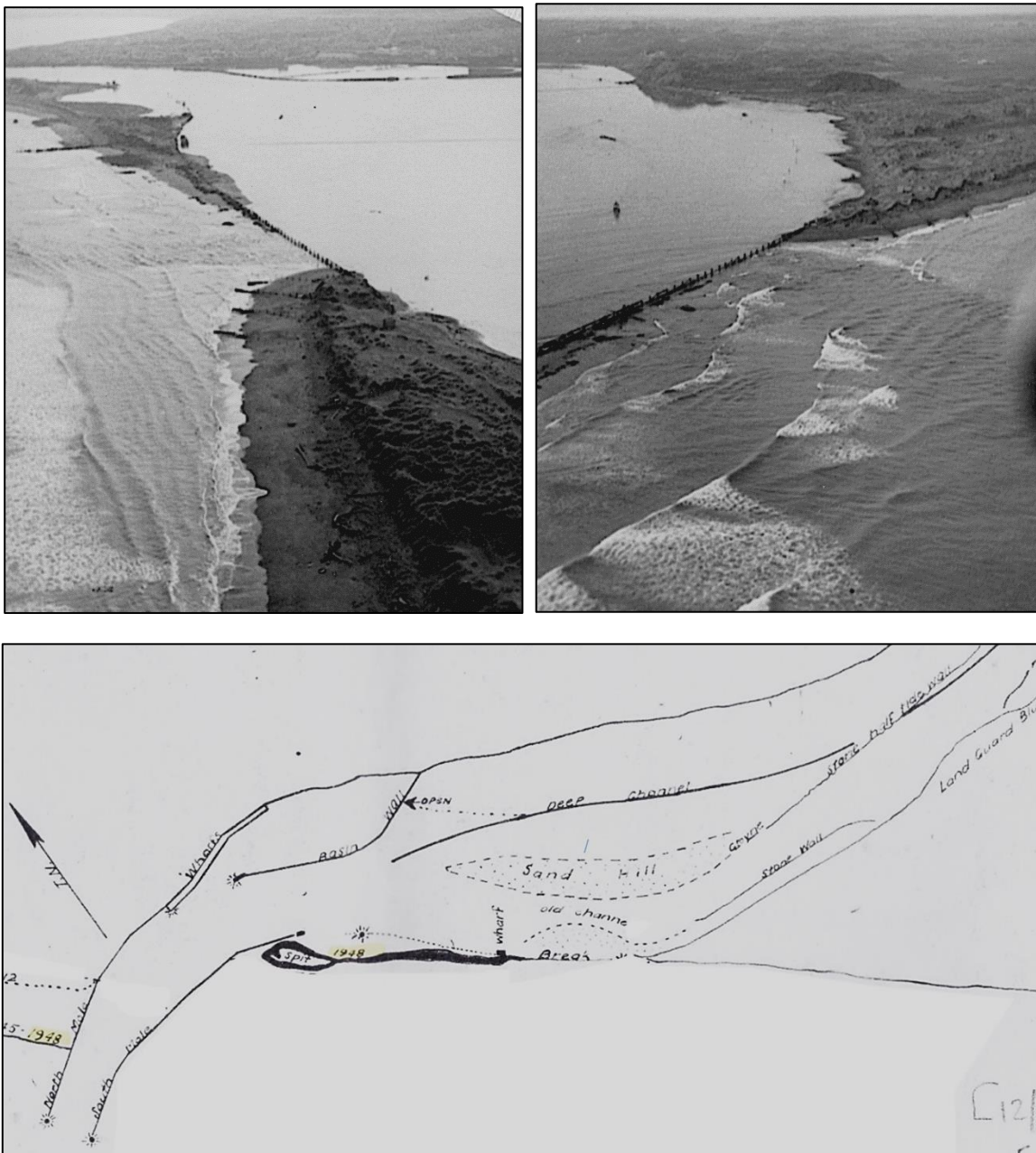
Figure 9 South Spit Breach on 5-7-1947 (upper photos) taken at high/ebbing tide and as sketched by Harbour Board staff in 1948 (lower) with surrounding morphological features referred to in the text having been marked.
