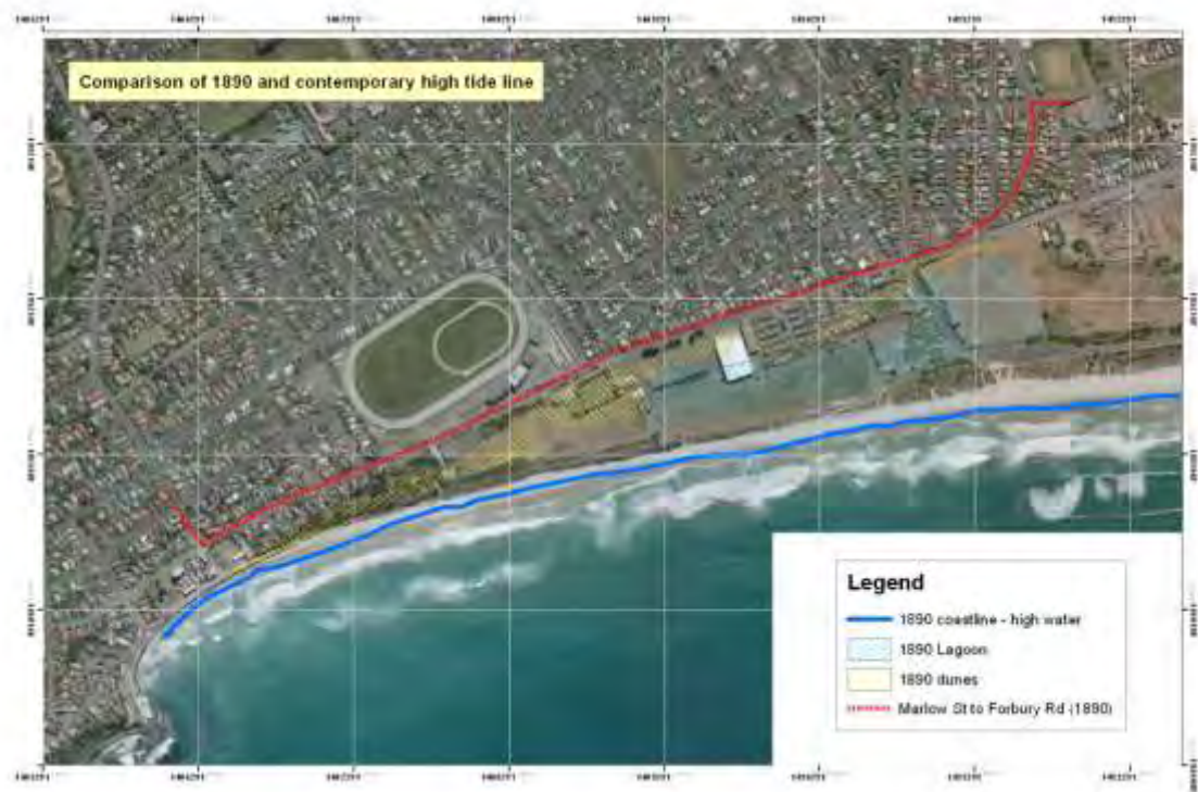
Figure 3-2 Comparison of the 1890 and present high tide line inferred as the difference between the dry and wet beach
