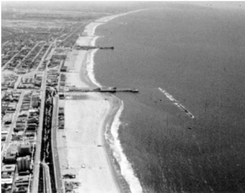
Figure 9-12 Example of an offshore emerged breakwater off the USA coastline (Source: CEM, 2006)
