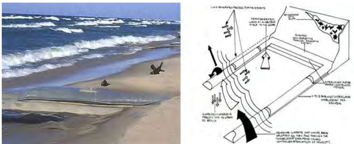
Figure 9-15 Schematic of an undercurrent stabilizer (Source: www.oceanusinternational.com )
