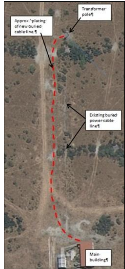
Figure 4: Aerial photograph showing the existing transformer pole and proposed route of the new underground power cable (copied from Ladley 2017).
