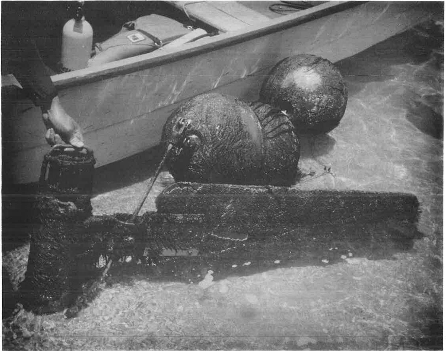
**Figure 1.** Bio-fouling on an Aanderaa RCM4 after a 2 month deployment in a tidal inlet.
