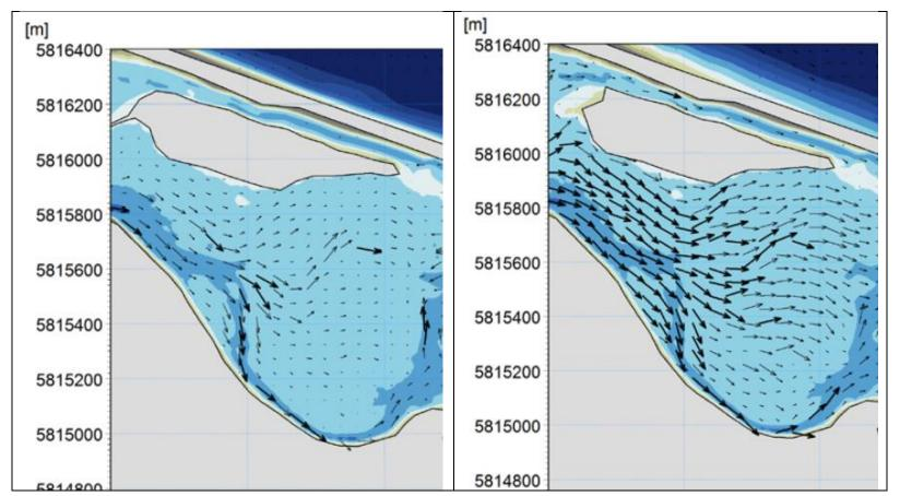
Figure 20: Residual sediment transport rates and directions within the estuary for the existing situation (top) and with the proposed re-diversion (bottom). The sediment residuals are those that occur during mean river flow over a neap-spring cycle. (Figures provided by DHI from their modelling reported in DHI, 2014. Transport rates are low and arrows have been scaled so that differences can be seen).
