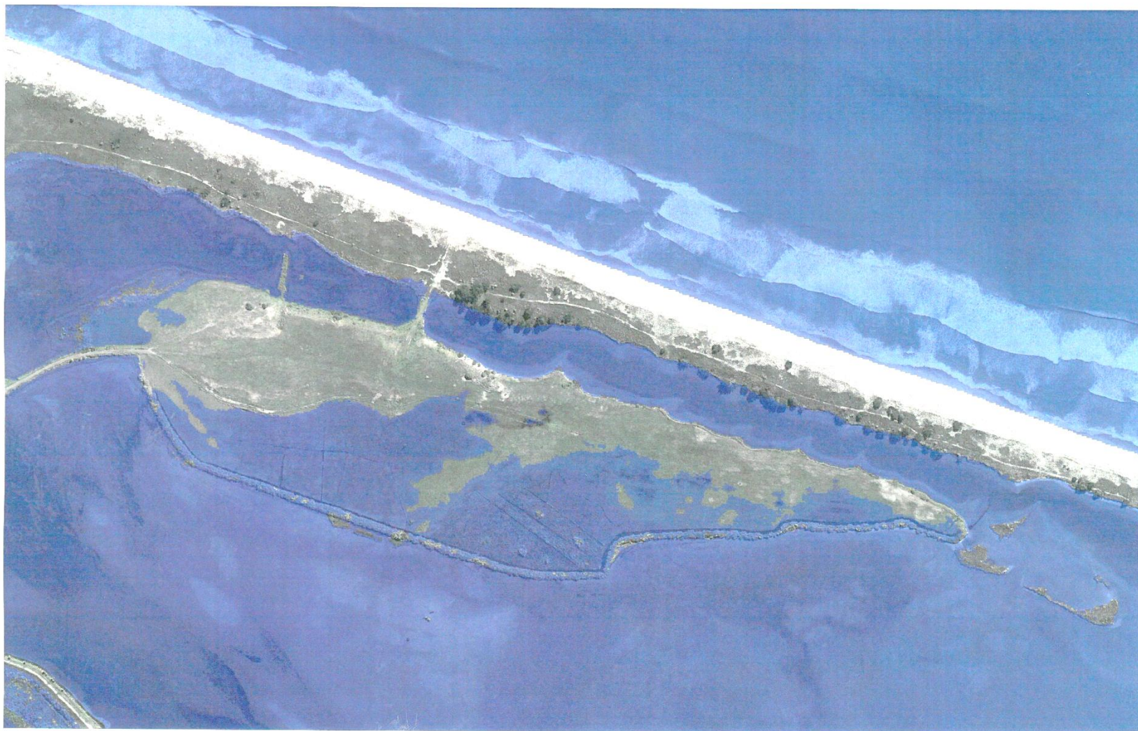
Figure 19: Likely maximum level of tidal inundation at spring high tide on Papahikahawai Is. once stopbanks and causeways are removed after re-diversion. [Inundation mapped at 1m above om RL Moturiki Datum]
