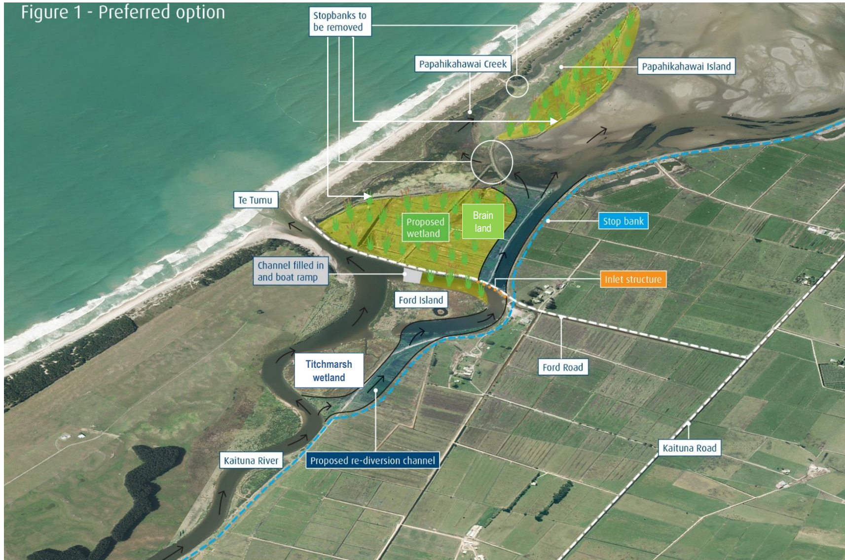
Figure 1: Graphic representation of the proposed re-diversion works and wetland restoration
