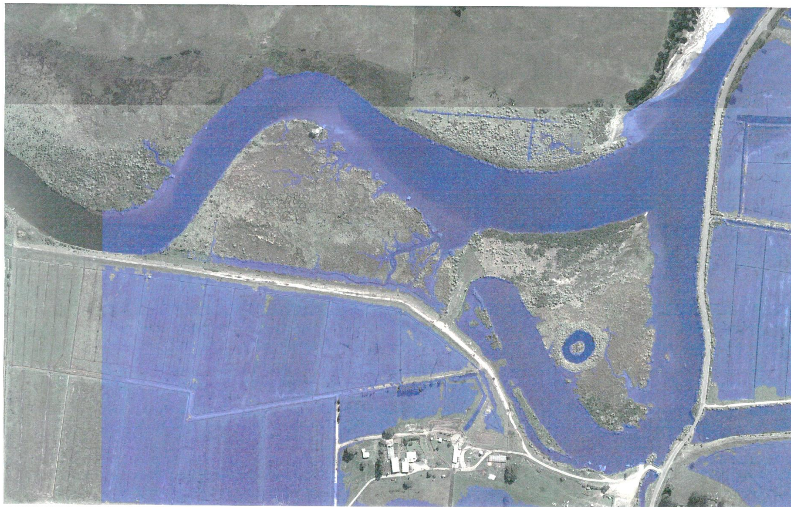
Figure 11: Likely level of tidal inundation at mean high tide on the Titchmarsh wetland and Ford Island after re-diversion. [Inundation mapped at 0.75m above om RL Moturiki Datum]
