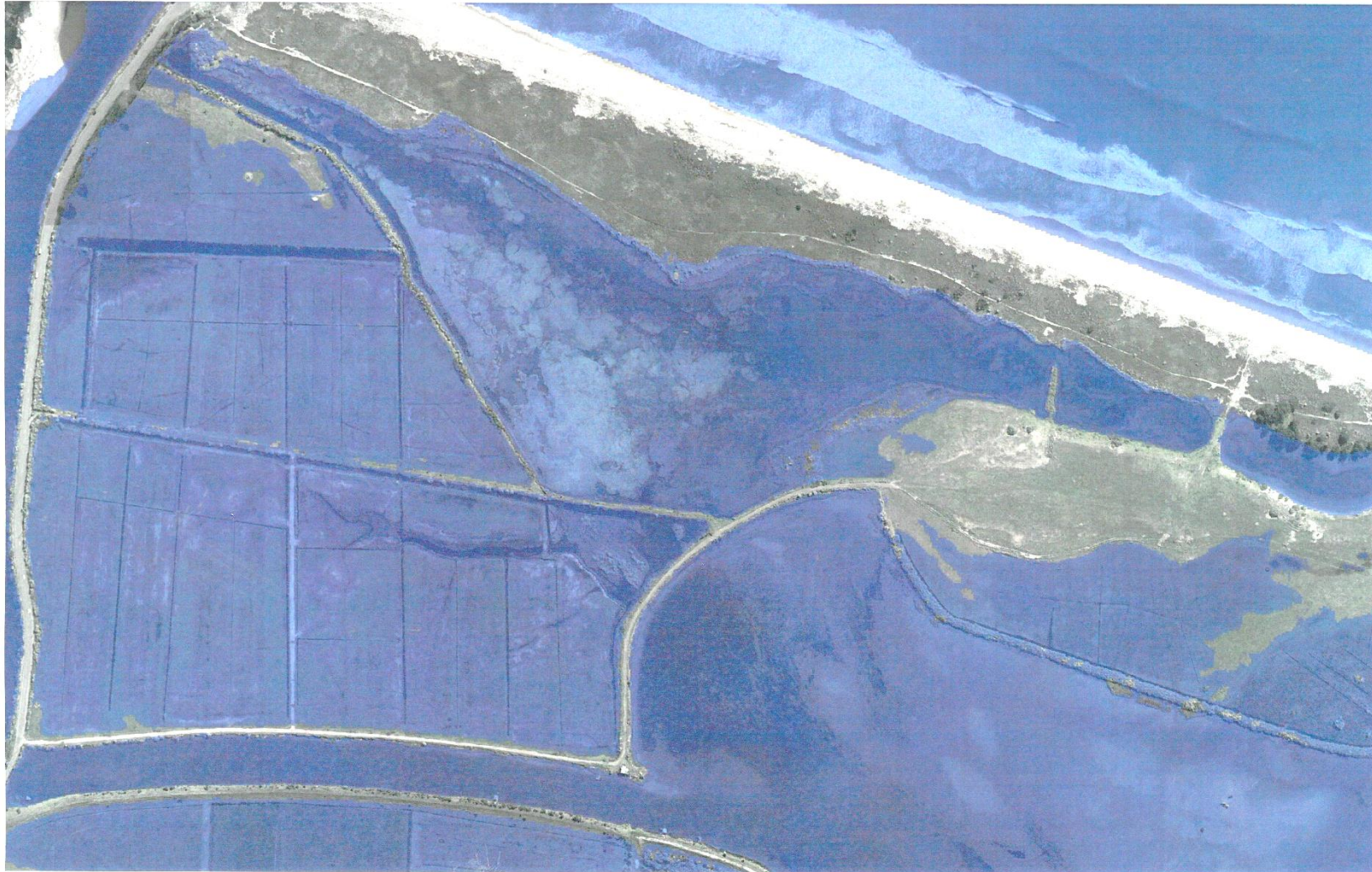
Figure 17: Likely maximum level of tidal inundation at spring high tide on the Brain land once stopbanks and causeways are removed after re-diversion. [Inundation mapped at 1m above om RL Moturiki Datum]
