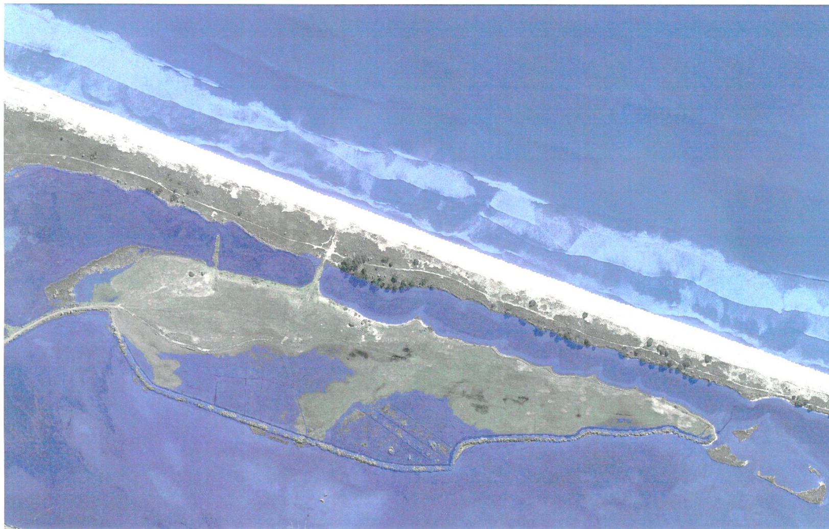
Figure 18: Likely level of tidal inundation at mean high tide on Papahikahawai Is. once stopbanks and causeways are removed after re-diversion. [Inundation mapped at 0.75m above om RL Moturiki Datum]
