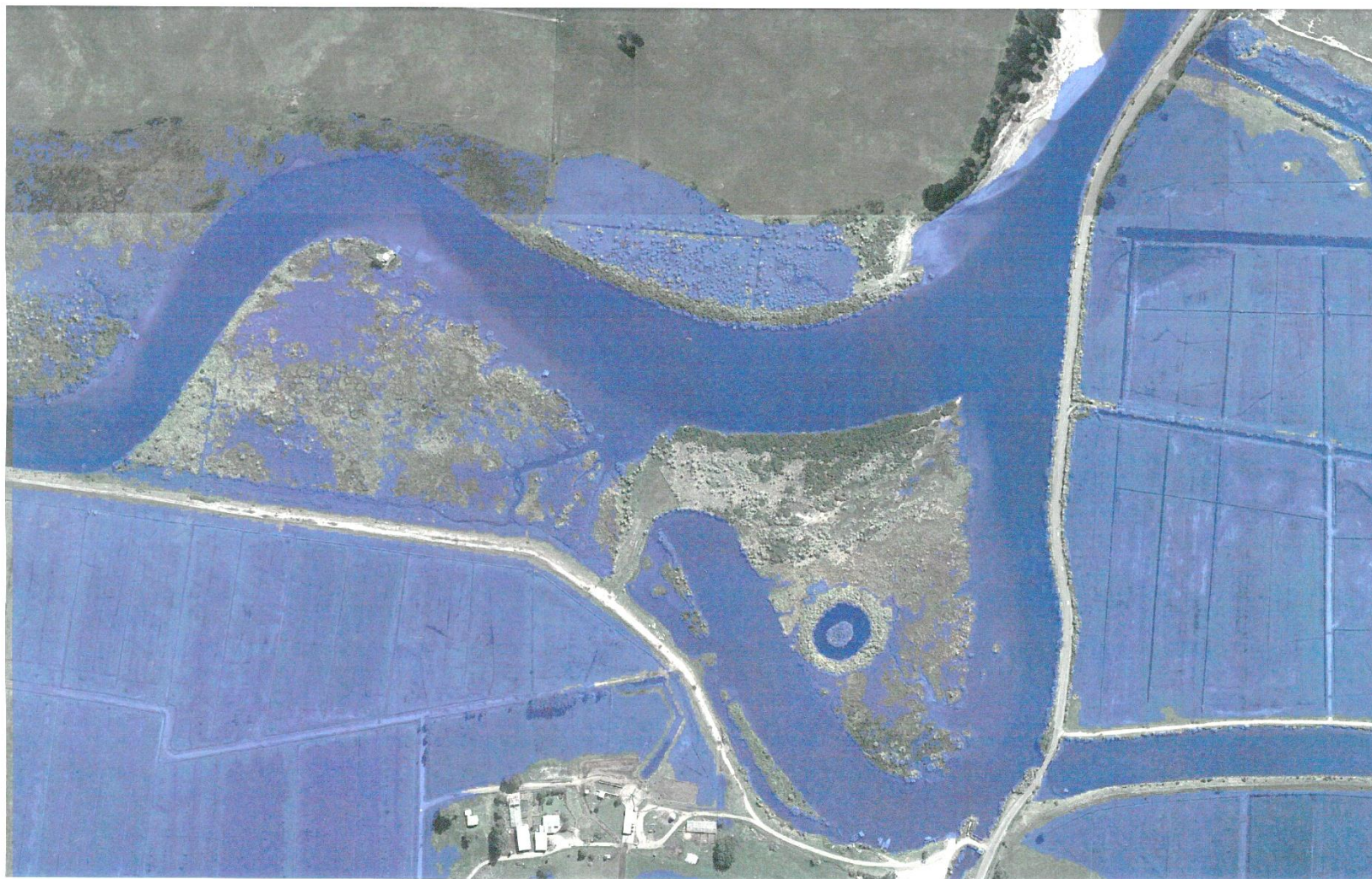
Figure 12: Likely maximum level of tidal inundation at spring high tide on the Titchmarsh wetland and Ford Island after re-diversion. [Inundation mapped at 1m above 0m RL Moturiki Datum]
