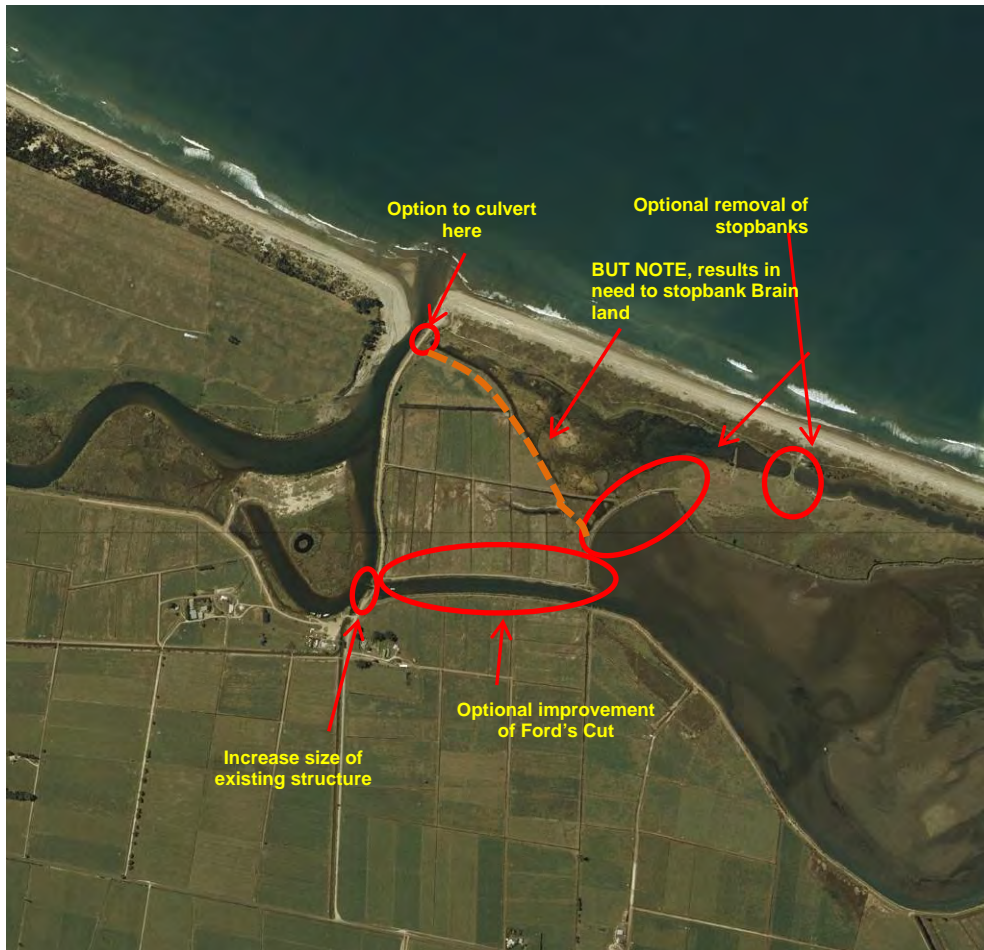
Figure 7 Low flow partial diversion.
