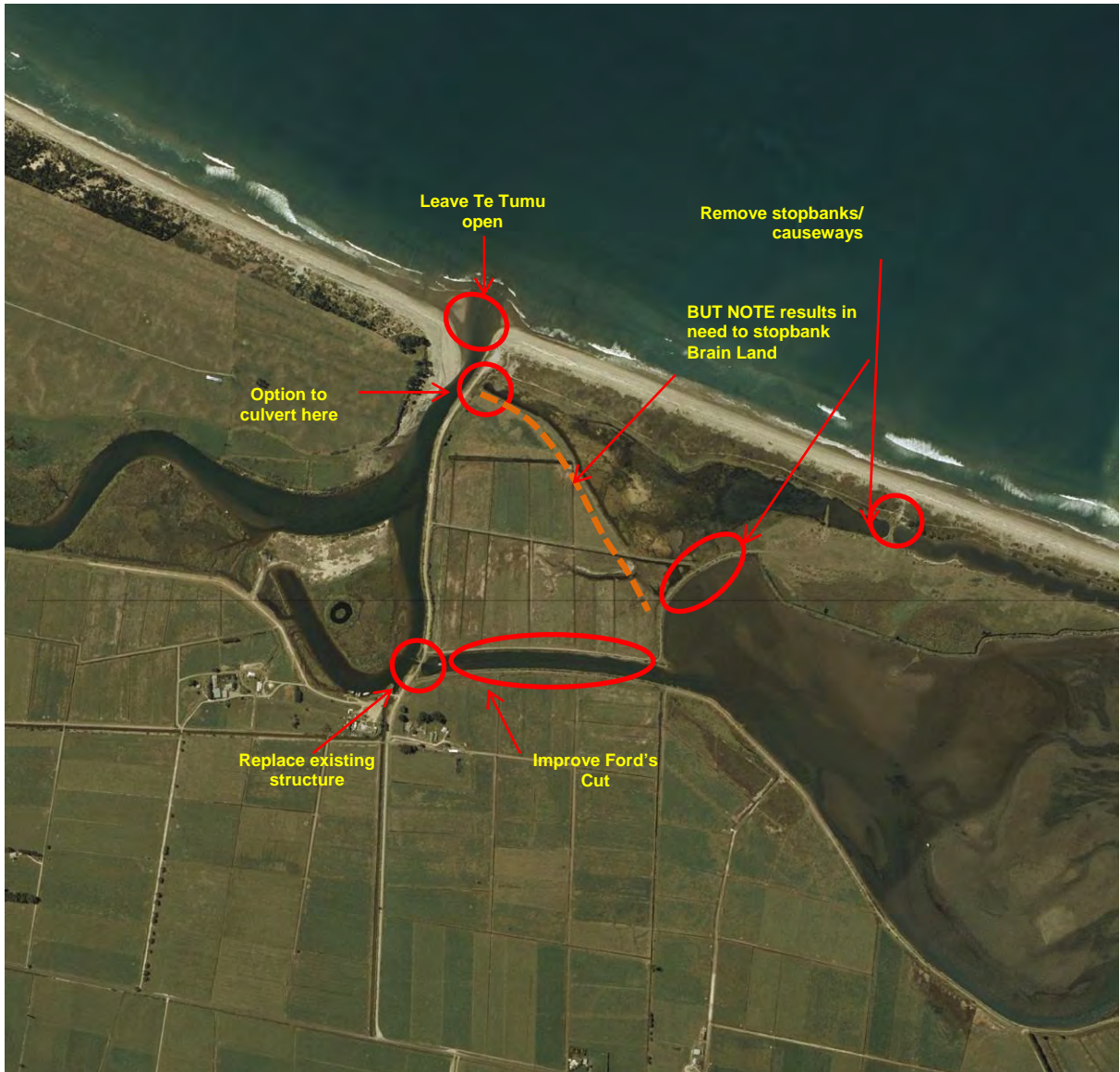
Figure 8 Maximum flow partial diversion.
