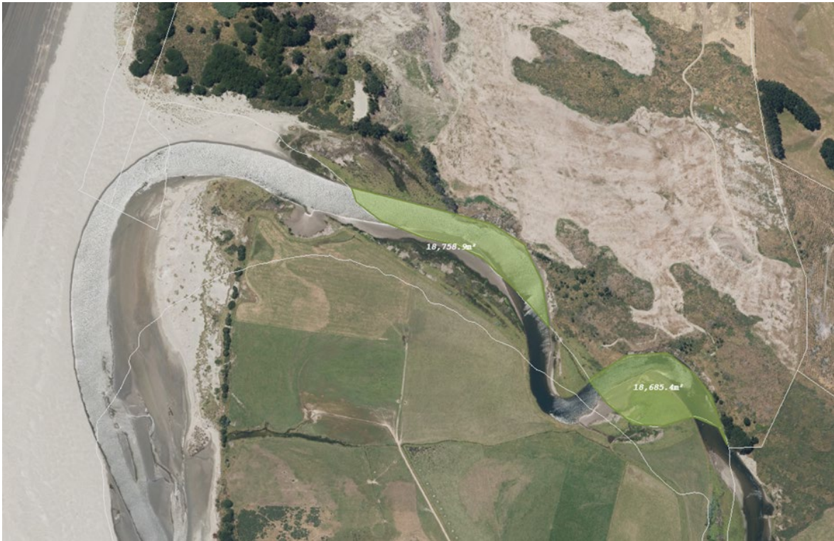
Figure 5: View of river margin of property showing (light green shading) the location and approximate area of bank erosion since 1975.
