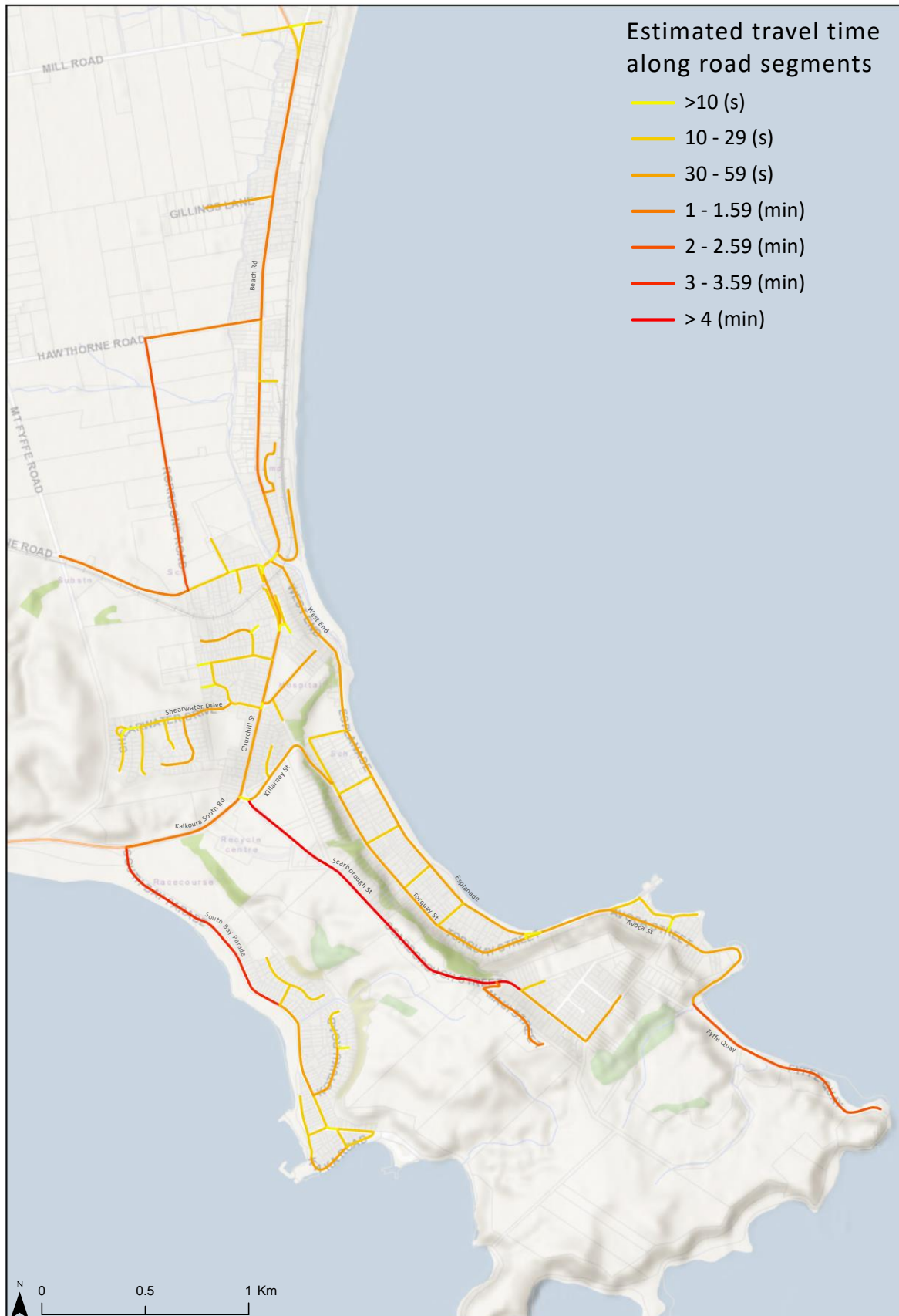
Figure 4.3-4: Map displaying predicted evacuation travel time along each road segment. Red represents greater evacuation time, yellow represents quicker time to travel along road segments.
