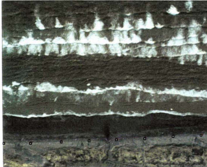
Figure 3.2 A vertical aerial photograph of a section of the study area taken on 20.1.99 from an altitude of 6000 feet. Ground control points used in the rectification procedure (section 3.2.4.1) are marked with small squares. These points are located at 100 m intervals along the foredune toe.
