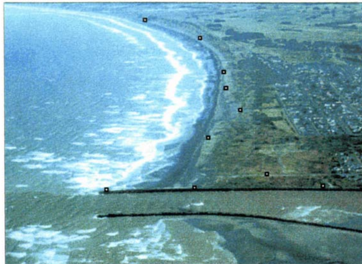
Figure 3.3 An oblique aerial photograph of the study area sampled on 9.1.93 from an altitude of 1500 feet. The small squares mark ground control points used in the rectification procedure (section 3.2.4.2). The Wanganui Rivermouth in the foreground marks the southeastern boundary of the study area and the most distant control point locates the northwestern boundary.
