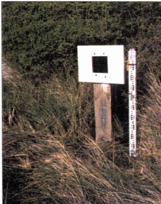
Figure 3.4 Field equipment used for oblique terrestrial photography. Figure A shows the camera with filter mount, lens hood, release cord, light bag and support tripods. This equipment is in operational position at the camera site which is ~3200 m alongshore from the rivermouth jetties, ~42 m above mean sea level and ~130 m landward of the foredune toe. Figure B shows a typical ground control marker located at the rear of the foredune.
