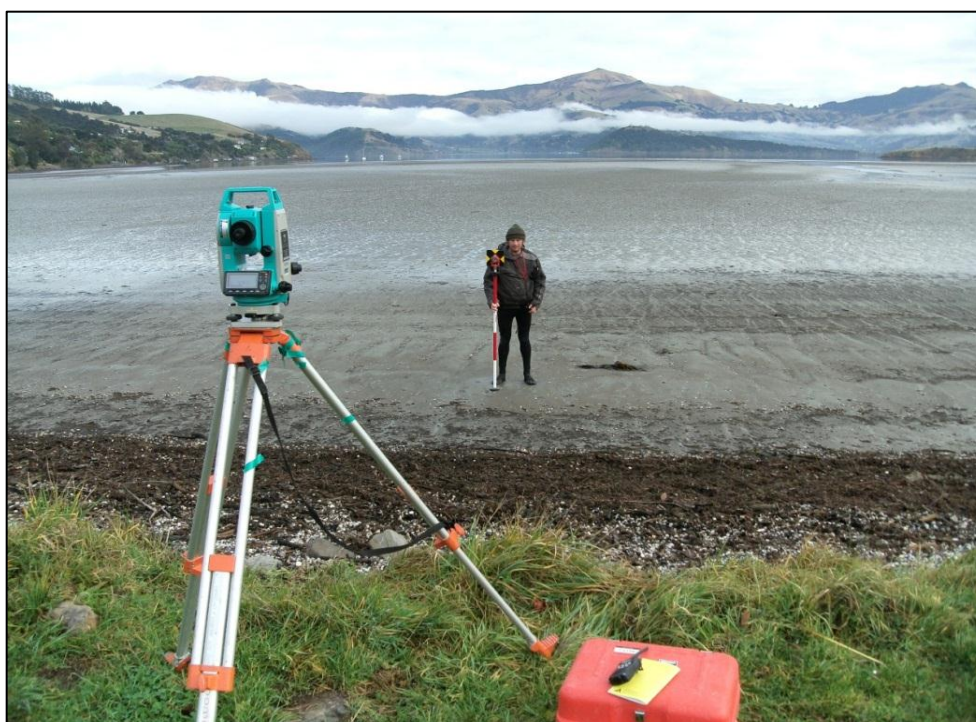
Figure 3.3: Sokkia 50RX Total Station set up in Takamatua Bay. Photograph by Doug Eaves.
