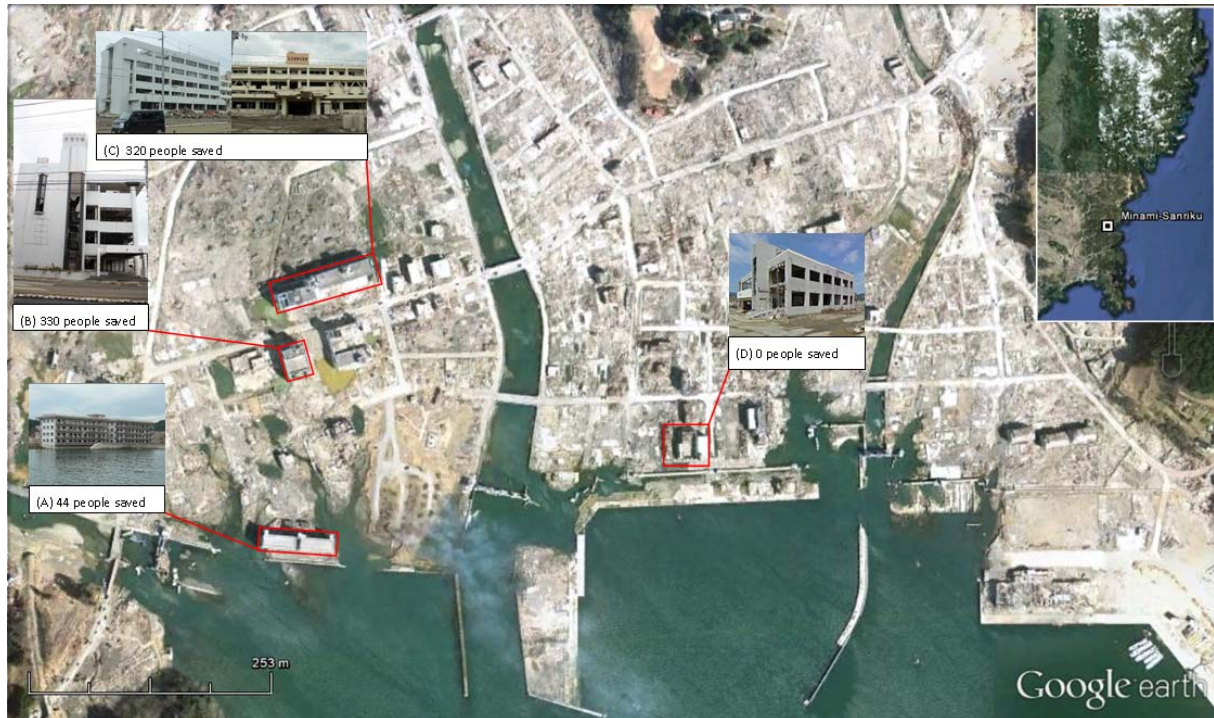
Figure 54 Locations of designated tsunami evacuation buildings in Minami-Sanriku Town: (A) Matsubara apartments; (B) Takano Kaikan building; (C) Shizugawa Hospital; (D) Fisheries Co-operative. Significant scour can be seen where seawater is encroaching around building (A) and to the east of building (D).
