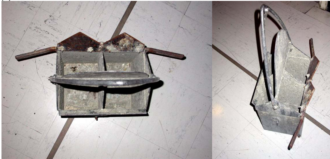
Figure 3 The box scoop used to collect sediment samples between 1.5 to 3 m below MSL (a) and the 0.3 m-wide, 0.2 m-tall and 0.3 m-long box dredge used to collect biological samples (b). Diagram by Justin Harrison and photo by G. Murphy.
