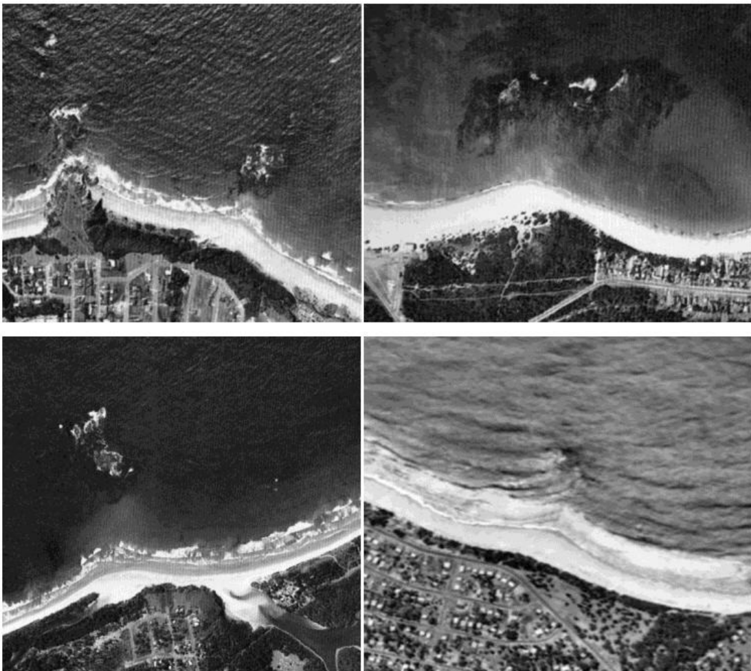
Figure 5. Natural coastal protection due to salient formation in the lee of offshore reefs in New South Wales, Australia. Clockwise from top left a) Sapphire Gardens to Emerald Beach, b) Toukey and Budgewoi, c) Conjola Beach and Ulladunlla, d) Woolgoola to Red Rock. (Source: Readers Digest, 1986)
