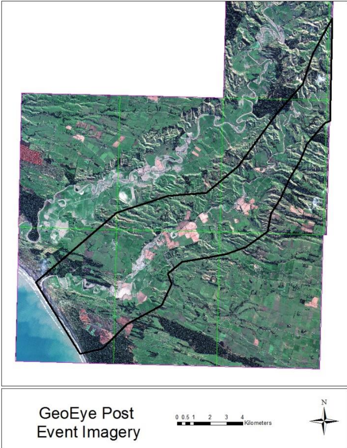
Figure 53. Mosaic of GeoEye-1 3 band imagery captured 12 July 2015. Black polygon defines the Turakina flood corridor of interest. Northwest of the lower Turakina Catchment, the floodplain of the Whangaeahu River is visible.
