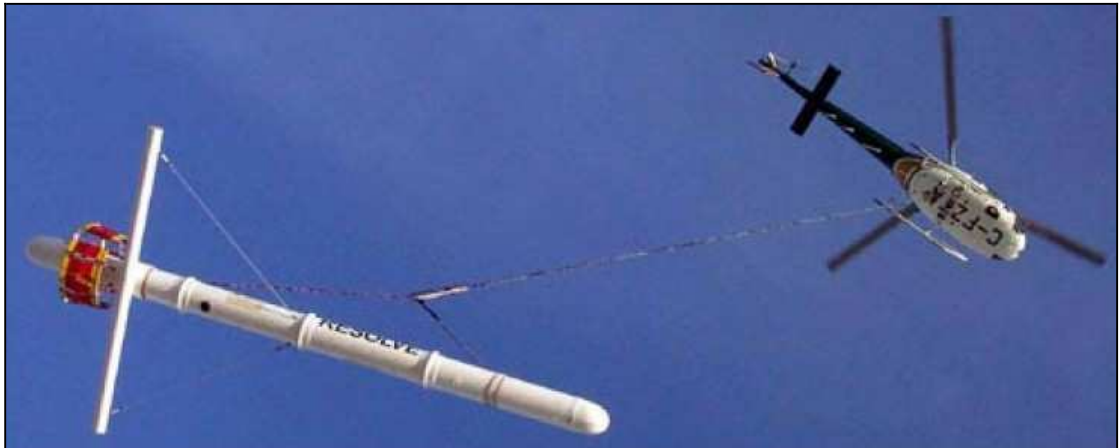
Figure 4.6 The helicopter and “bird” used for the airborne EM survey (provided by Ian Brown Associates).
