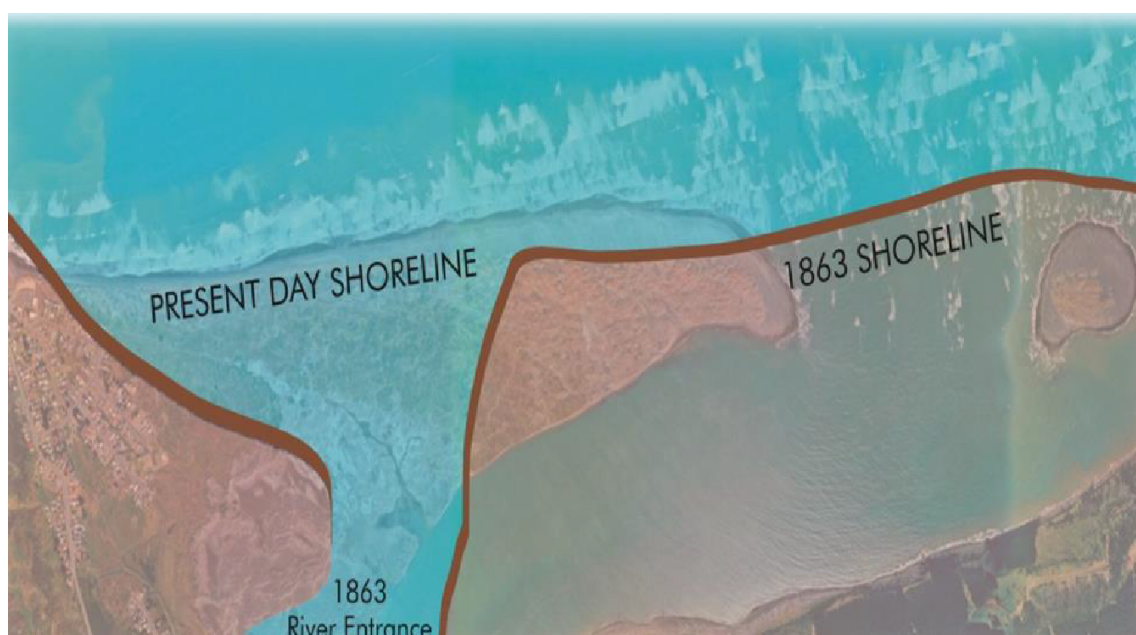
Figure 1: Diagram illustrating overall shoreline change at the Waikato River entrance between 1863 and the present.
