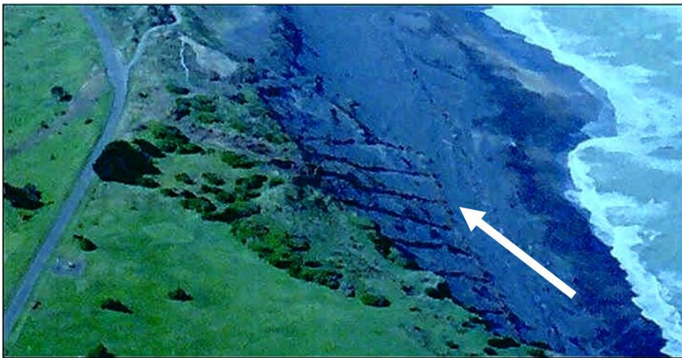
Figure 7 Upper photo (A) shows sand stabilization works in the eroding foredune area (NB C in Figure 6) where pine thinnings were placed in gullies and orientated across the path of the prevailing wind (arrow), with marram grass planted within the intervening spaces (photo 1988). In the northern area (lower photo B) sand instability was wide-spread and pine thinnings were used to erect rectangular fencing with marram planted in between (photo 1992).
