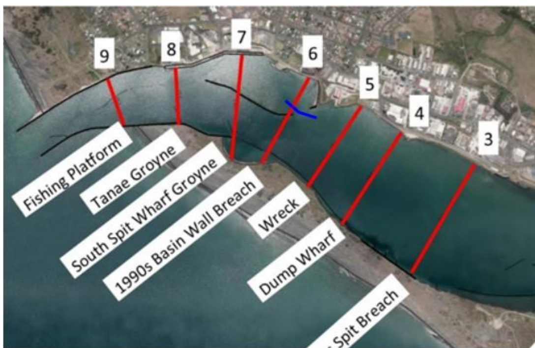
Figure 3 Section locations (red lines), numbers and names. Black lines locate river control structures. (source Figure 15, Baseline Study 2016). Blue line is transect sampled in Figure 5 to compare breach bed levels.
