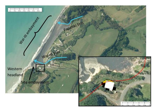
**Figure 1** Wai-iti Beach features and site (inserted) where the existing building is shown white, proposed modifications in black with proposed deck in yellow. The seaward property boundary is depicted by the black dash-dotted line, while the red line defines the current Area Susceptible to Coastal Erosion (ASCE) as defined in T&T (2018). 2012 aerial photo supplied by LINZ
