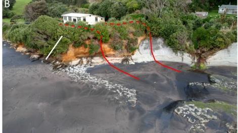
**Figure 2** Southern headland is depicted in photo A and the "site-embayment" fronting the Taylor property in photo B which also shows survey transects (red line) and the vegetated bank used to determine the stable slope angle for volcanic ash is marked by the white line (Photos taken on 2-9-2018)
