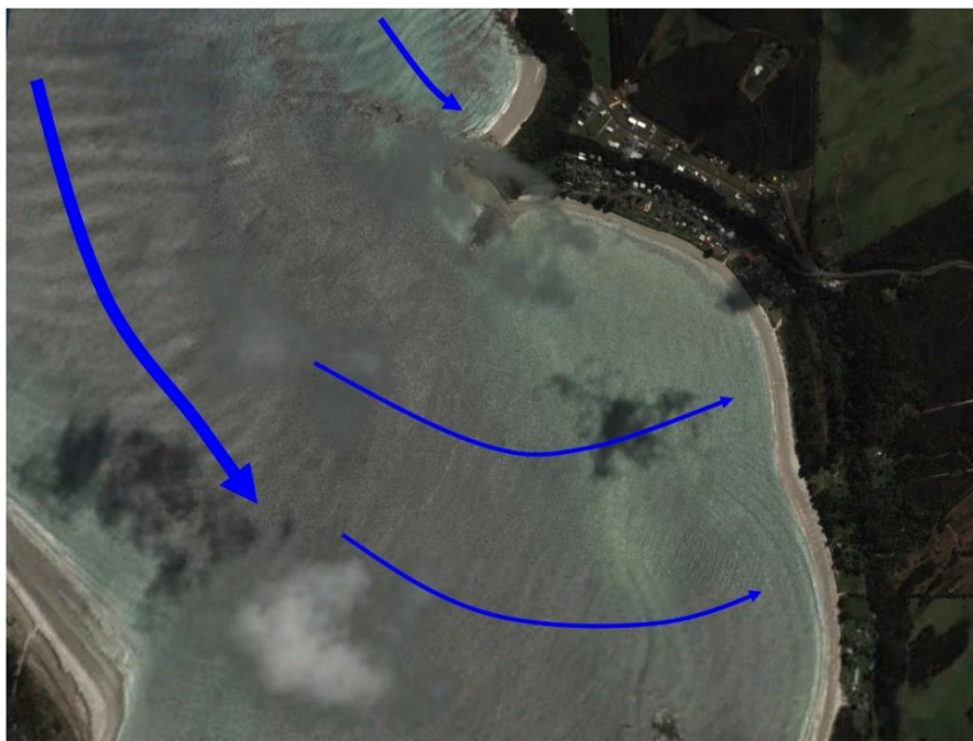
Figure 5 Wave transformation during propagation into the estuary. Note the dampening effect of the reefs off Kotiatia point and the particularly sheltered Rangiputa shoreline Image from Google Earth 2012
