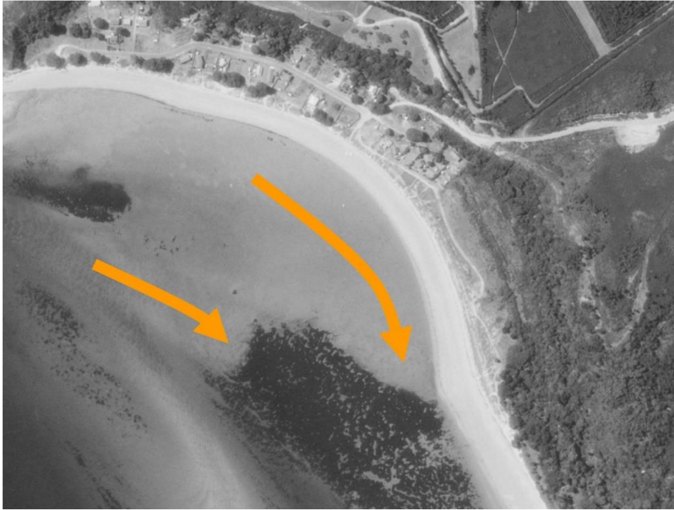
Figure 7 Sediment wave (lighter area) migrating to the south east (arrowed) over (smothering) a sea grass meadow (dark area). 1984 aerial photo
