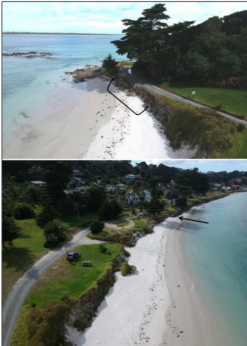
Figure 9 Wilkinson Beach viewed to west (top photo) with the rocky headland (Kotiatia Point) in the distance and the section of threatened access road bracketed. Southern view (bottom photo) shows Wilkinson Reserve in the foreground and the Rangiputa settlement and seawall in the distance (beyond arrow). CSL 2018 aerial photos
