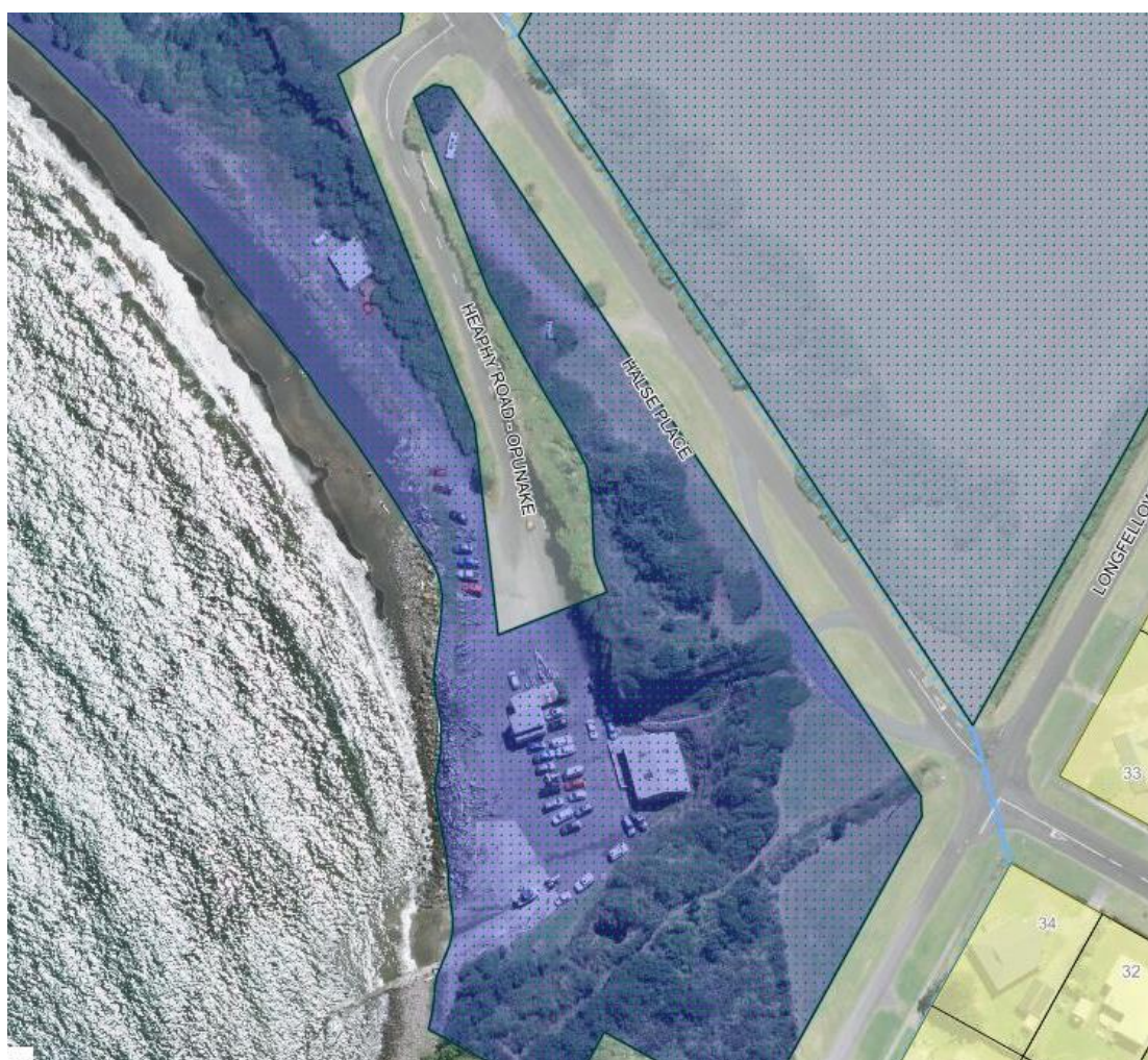
Council land is purple, roading reserve is shaded grey, coastal protection zone is blue line.
