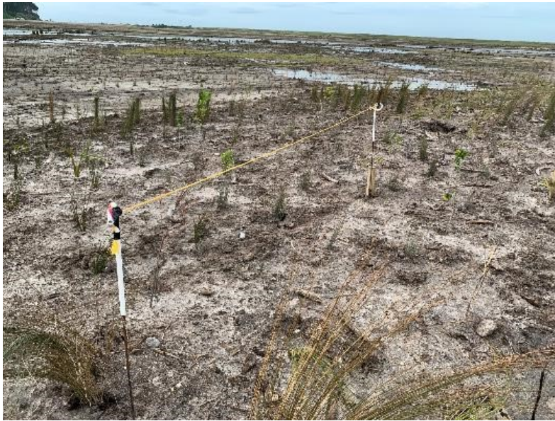
Two pig tail standards with connecting cord at a fixed radius of 2.5m or 5m was used to sample the planted natives within bounded circular plots around a centrally located wooden plot peg.
