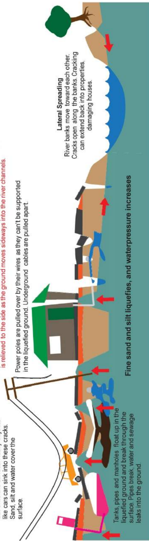
Figure 2.1 Schematic representation of liquefaction and its effects (Institution of Professional Engineers of New Zealand (IPENZ) Liquefaction fact sheet).
