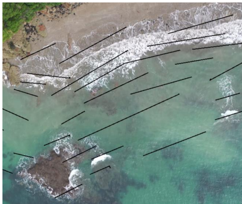
Figure 12: Image of the interim stage in the GIS wave refraction analysis. This is an example of line features being drawn on top of wave crests to track the wave's movement and patterns.
