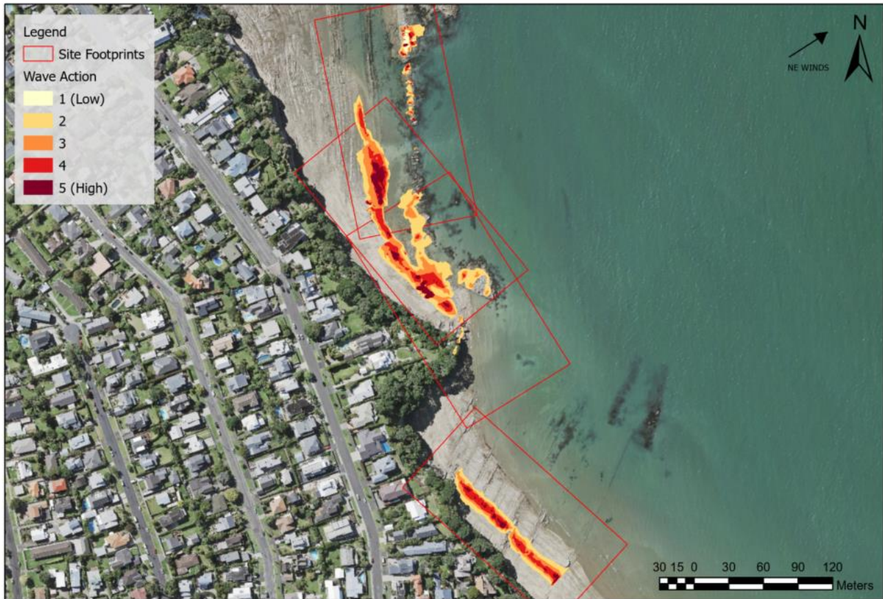
Figure 16: Vector results from the Image time stack - wave energy analysis taken at the study location (Narrow Neck). Map displays the spatial distribution of wave energy dispersion along the coastline as well as the occurrence of the wave action (Low to High scale of wave action).
