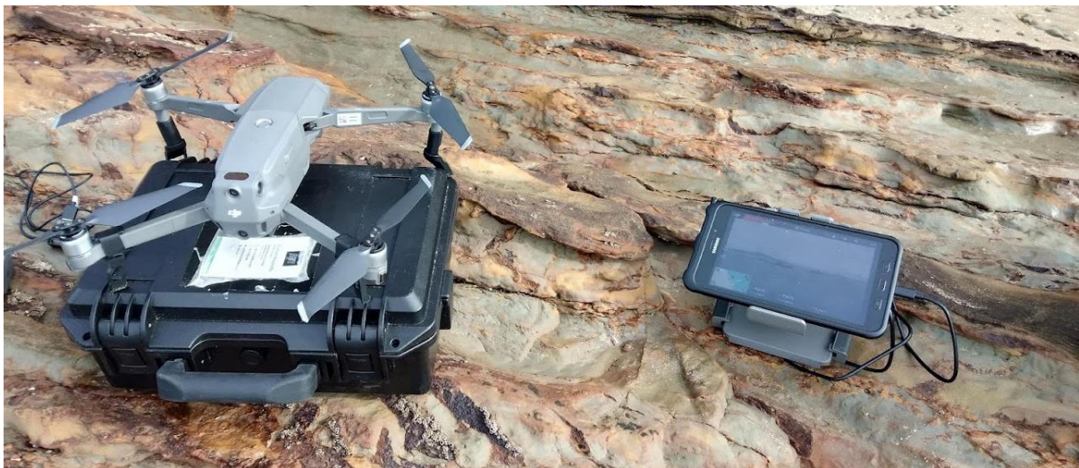
Figure 7: Image of the DJI Mavic 2 Pro UAV and mobile device that was operated on site to collect the FMV data.
