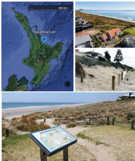
Figure 12- Location of Papamoa East, NZ, displaying the close proximity of coastal development to the coast, the coastal erosion on the coastal sand dunes in front of these areas of residential development and how dune plantings have successfully restored the dune system in Papamoa East
