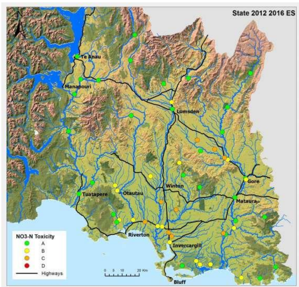
Figure 6-1: Nitrate-N in surface waters categorised according to the NPS-FM National Objectives Framework attribute states for toxicity to aquatic life. Annual median concentrations indicated by green (A) are \leq 1 mg/L; yellow (B) are 1-2.4 mg/L; orange (C) are 2.4-6.9 mg/L; and red (D) are >6.9 mg/L. Map from Hodson et al. (2008) and based on data from 2012-2016.
