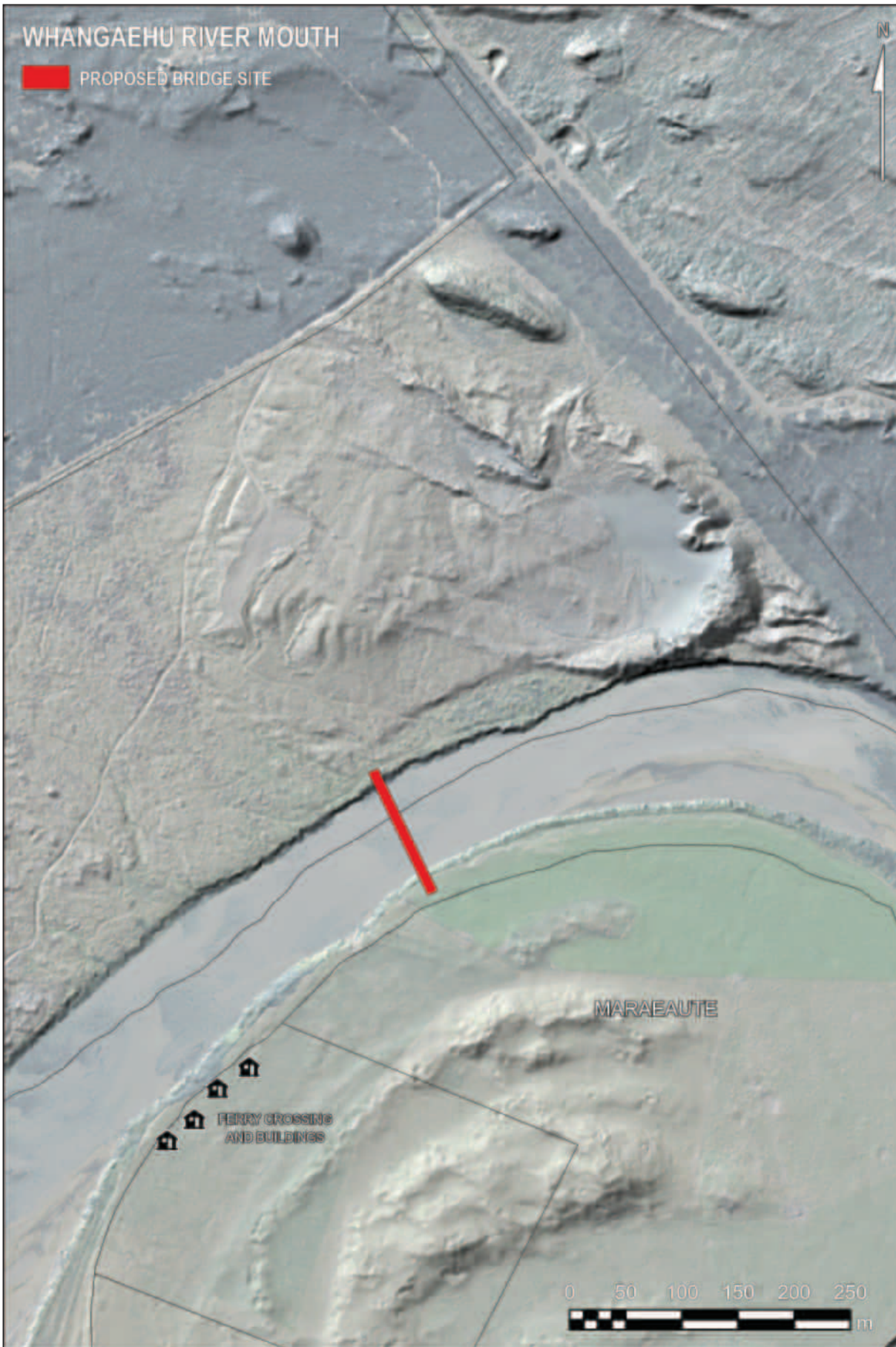
Figure 3: Detail of proposed pedestrian swing bridge location, showing differences in the stable (true left bank) and unconsolidated (true right bank) dune topography, historic place names and structures.
