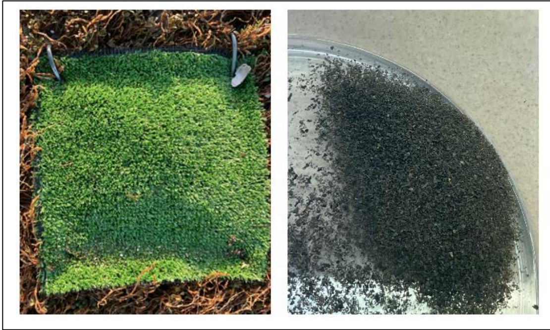
Figure 5.2: Left: 25 x 25 cm sediment mat after inundation event; right: black plastic particles from mat.
