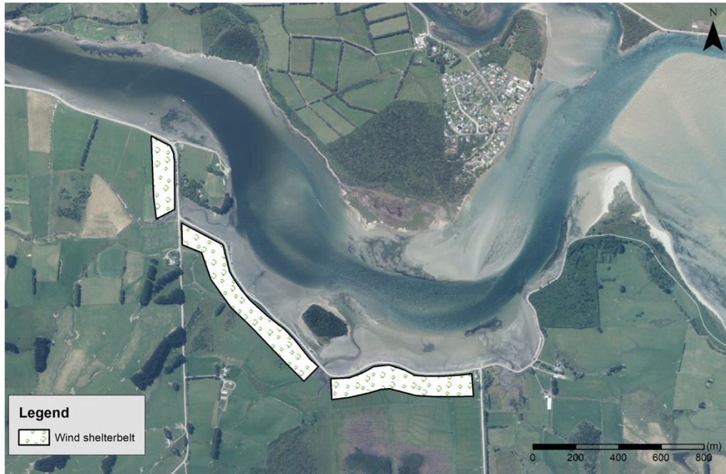
Figure 6.11: Potential shelter belt locations at Hinahina. Shelter belt is ~100 m wide and would reduce wind speed from south and south-westerly winds.
