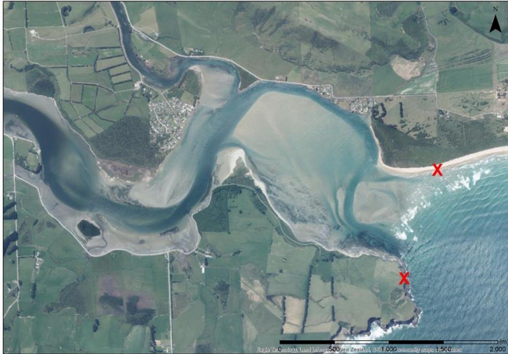
Figure 4.3: Locations of measurement for VLM for the NZ SeaRise: Te Tai Pari O Aotearoa programme. Red X's mark the locations of the North and South VLM indicators. VLM for the north is 1.06mm/yr, and the southern VLM is 1.67 mm/yr, the average of the two locations (1.37 mm/yr) was used for calculations.
