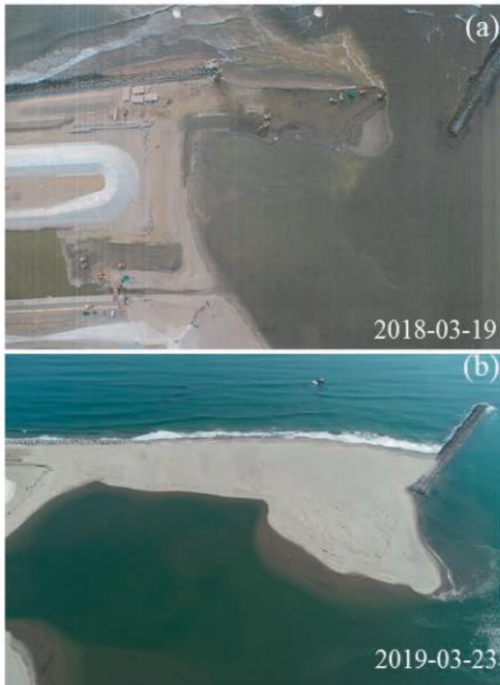
Figure 6.4: Aerial images of during and after sand nourishment of the sandspit at Naruse River, Japan (Nguyen et al. , 2019).
