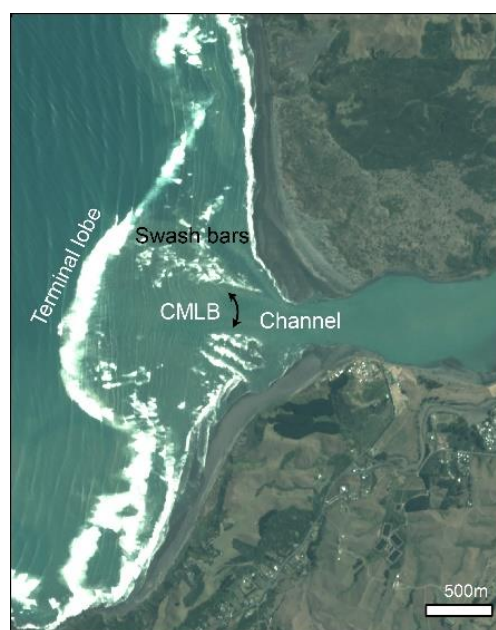
Figure 2 True colour PlanetScope Ortho Tile image of the Raglan ebb-tidal delta captured 24-Feb-2019 showing the main channel, swash bars, channel margin linear bars and breaking on the terminal lobe ( H_s = 3.02 m and water level = 0.97 m).
