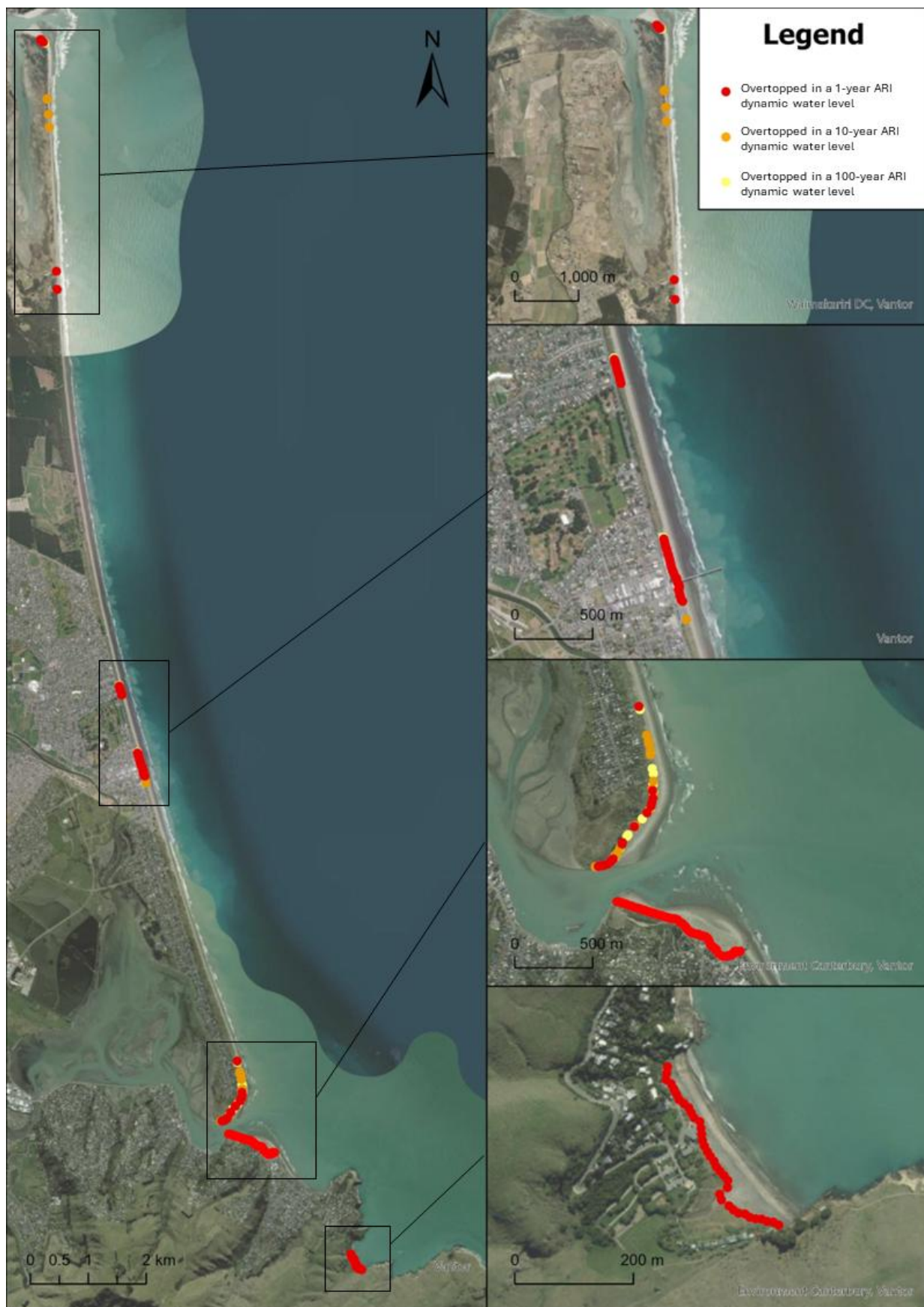
Figure 3-7: Locations along the shoreline where the current dune crest could be overtopped by runup water levels (e.g. dynamic overtopping) in a 1-year ARI (red), 10-year ARI (orange), or 100-year ARI (yellow).
