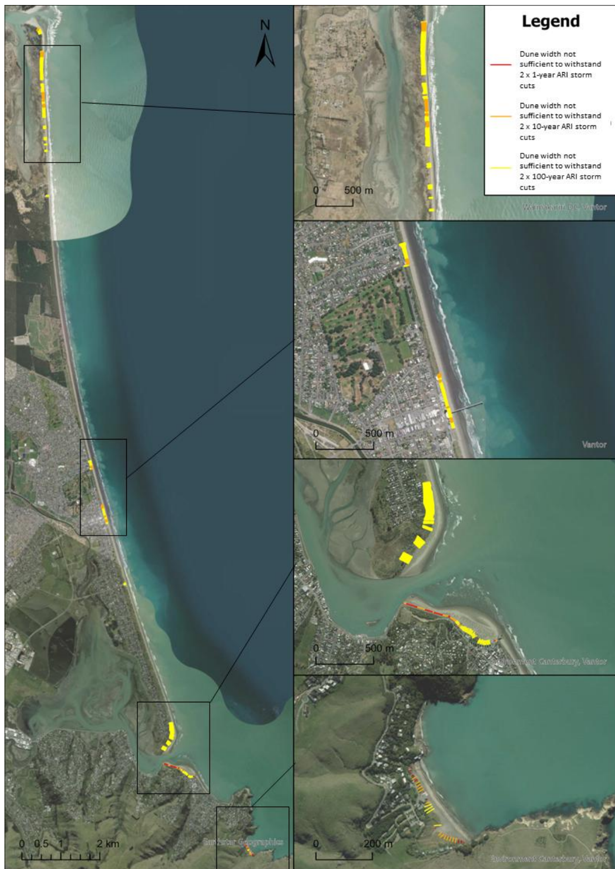
Figure 3-6: Mapping results of the dune width analysis, showing areas susceptible to dune breaching from storm cut erosion.
