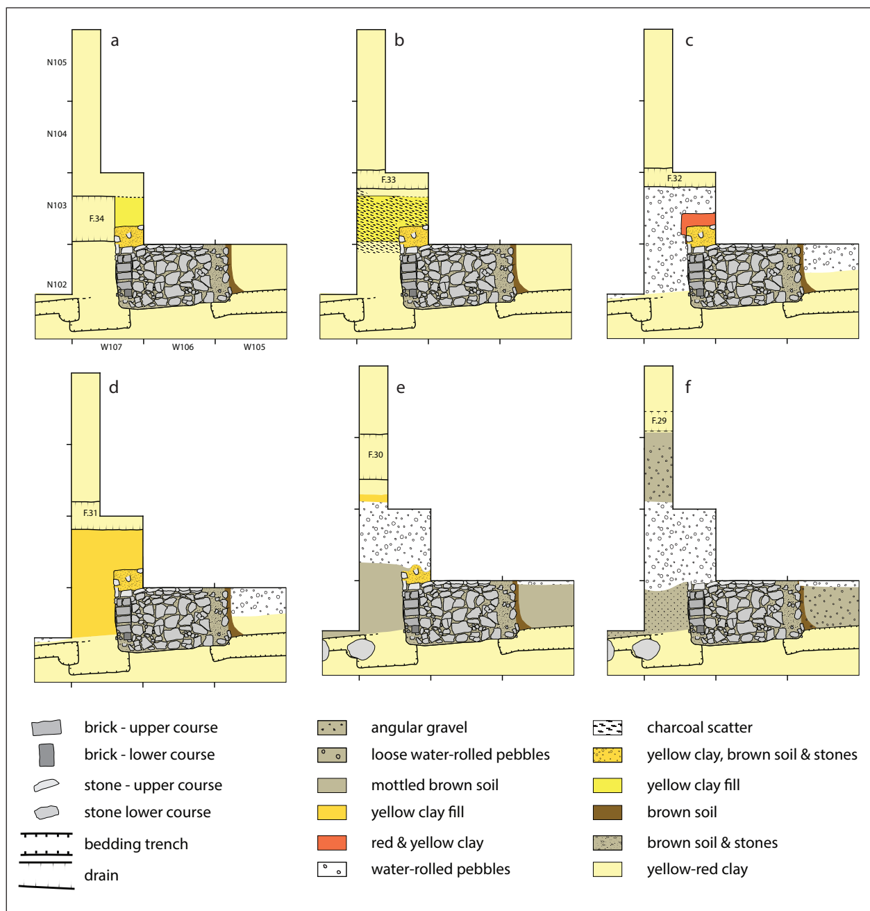
Figure 24. Construction sequence at northwest corner of chimney
