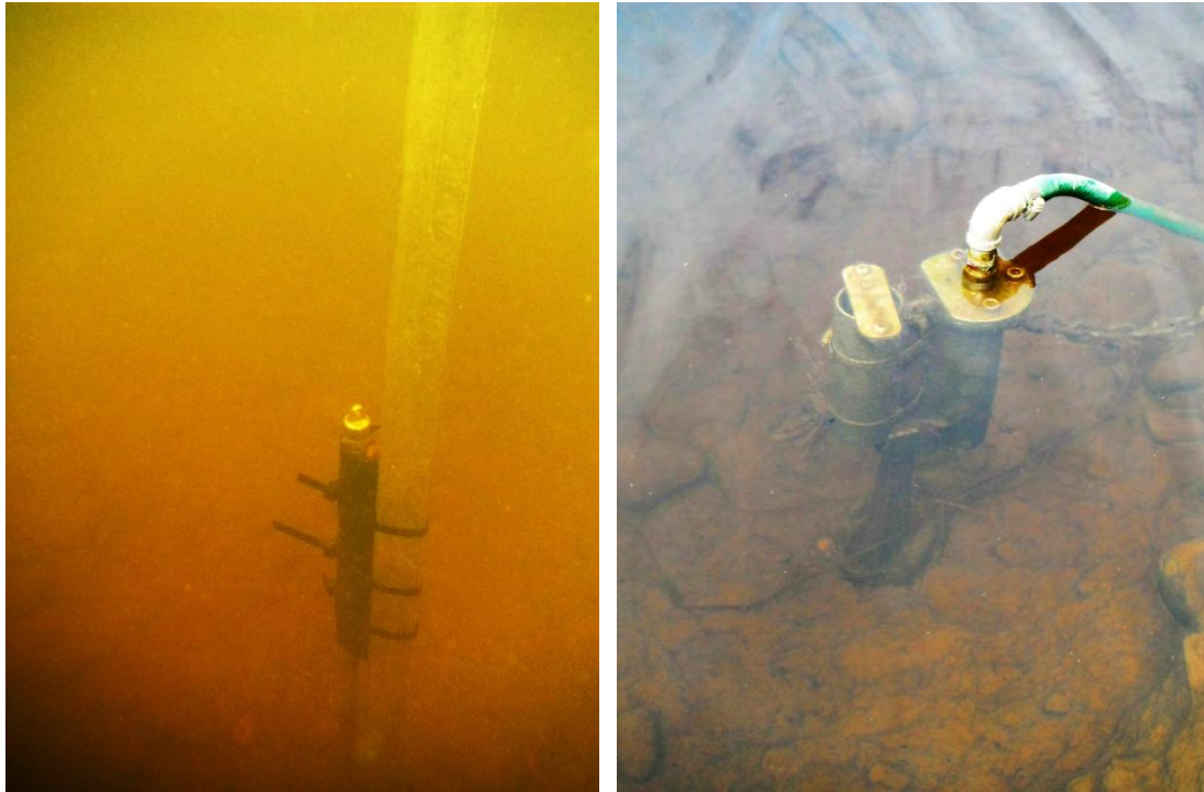
Figure 5.3. To the left is the short term water level, temperature and salinity recorder fastened to a steel pole and to the right is the long term water level, temperature and conductivity recorders, both encapsulated in steel brackets and fastened on either side of a steel pole (05/03/2012).
